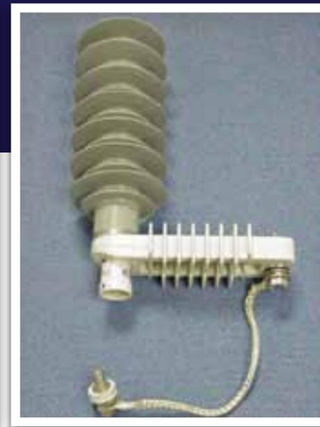
Fig.5 GLD operating prematurely creates a difficult scenario for the linesman
