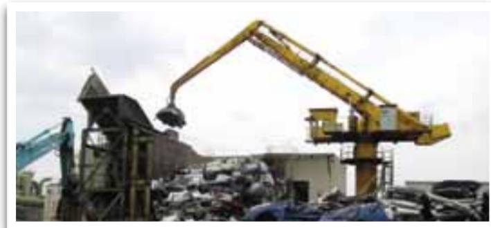
Figure 1: Typical Metal Shredder
