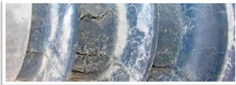
Fig.19: Severe erosion and tracking observed on insulator product 11-31.
