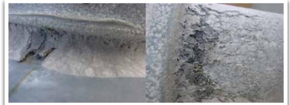
Fig. 14: Material erosion observed in the sealant at the end-fitting on high voltage line post insulators tested at KIPTS.
