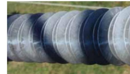
Fig.6: Chalking observed on the EPDM insulator tested at the Clansdale tower in Natal.
