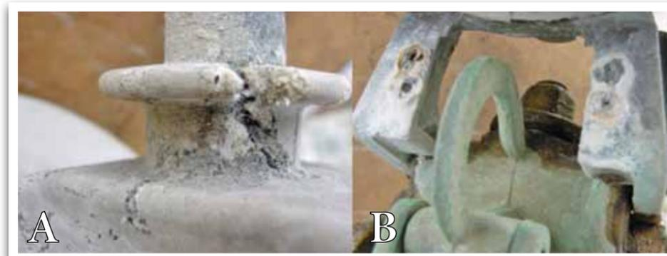
Fig.16: Severe material erosion (a) and metalware corrosion (b) as found on two of the LSR cut out fuses (units 22-20 and 22-21) tested at KIPTS.
