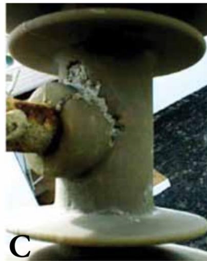
Fig.2: (a) Silicone rubber insulator after 8 months energised at KIPTS, (b) Field aged Cycloaliphatic cut-out fuse, (c) Cycloaliphatic cut-out fuse after natural ageing test at KIPTS.
