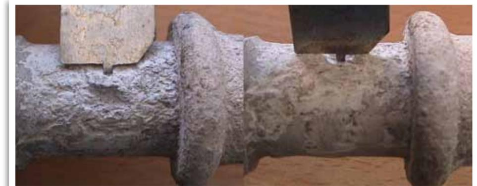
Fig.3: Erosion depth is measured with a special little tool to determine if it is deeper than 2 mm. The insulator shown was defined as failed due to severe erosion present.
