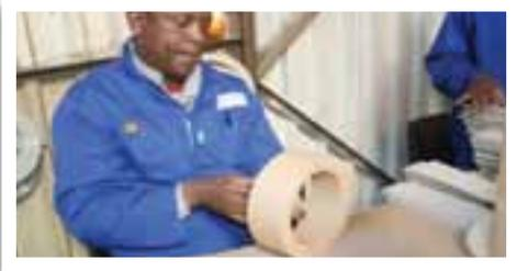
Copper wire is then wound around the core, depending on the specified burden, ratio and accuracy required.
