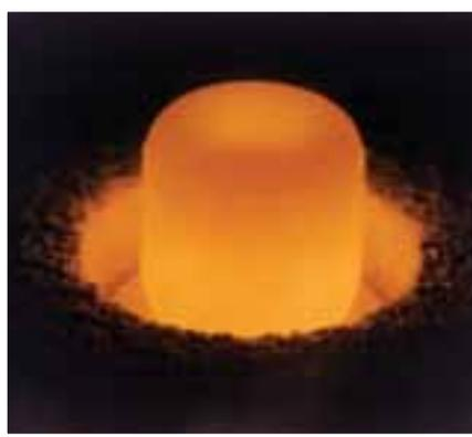
Figure 3 - Decaying Plutonium fuel pellet: providing energy through heat.
