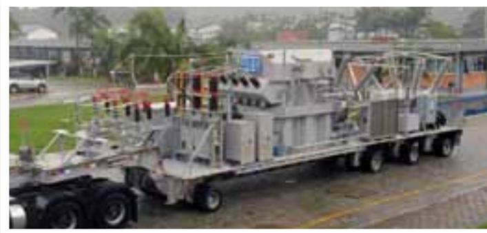
*A WEG 30 MVA 138/69 34.5/13.8 kV mobile substation with an hydraulic goose neck and articulated rear wheels to accommodate tough terrain and any logistic challenge.*
