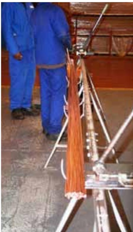
*Solid copper conductors wrapped together*
