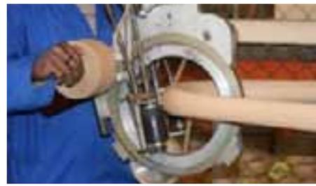
*Insulating tape being wrapped onto copper*
