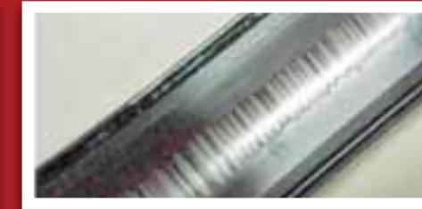
*Damaged Grease & Bearing fluting, "washboard" pattern on bearing race*
