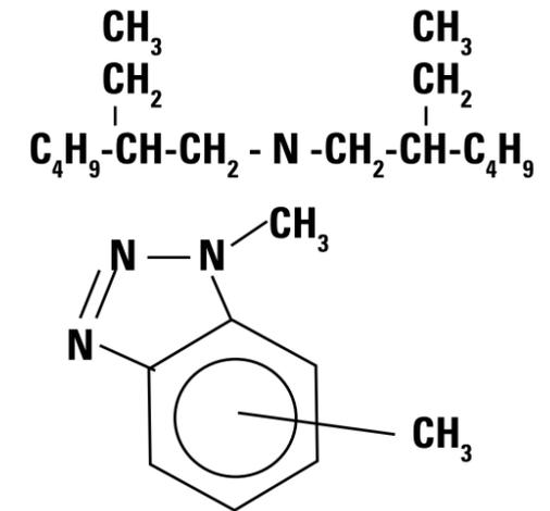
Figure 1: Chemical structure of N-Bis (2-ethylhexyl)-aminomethyl-tolutriazole used as metal passivator
