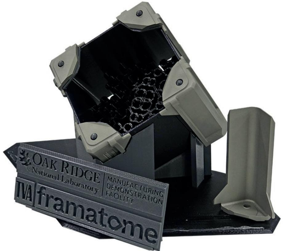
*Additively manufactured channel fasteners for Framatome's boiling water reactor fuel assembly. (Source: Oak Ridge National Laboratory)*
