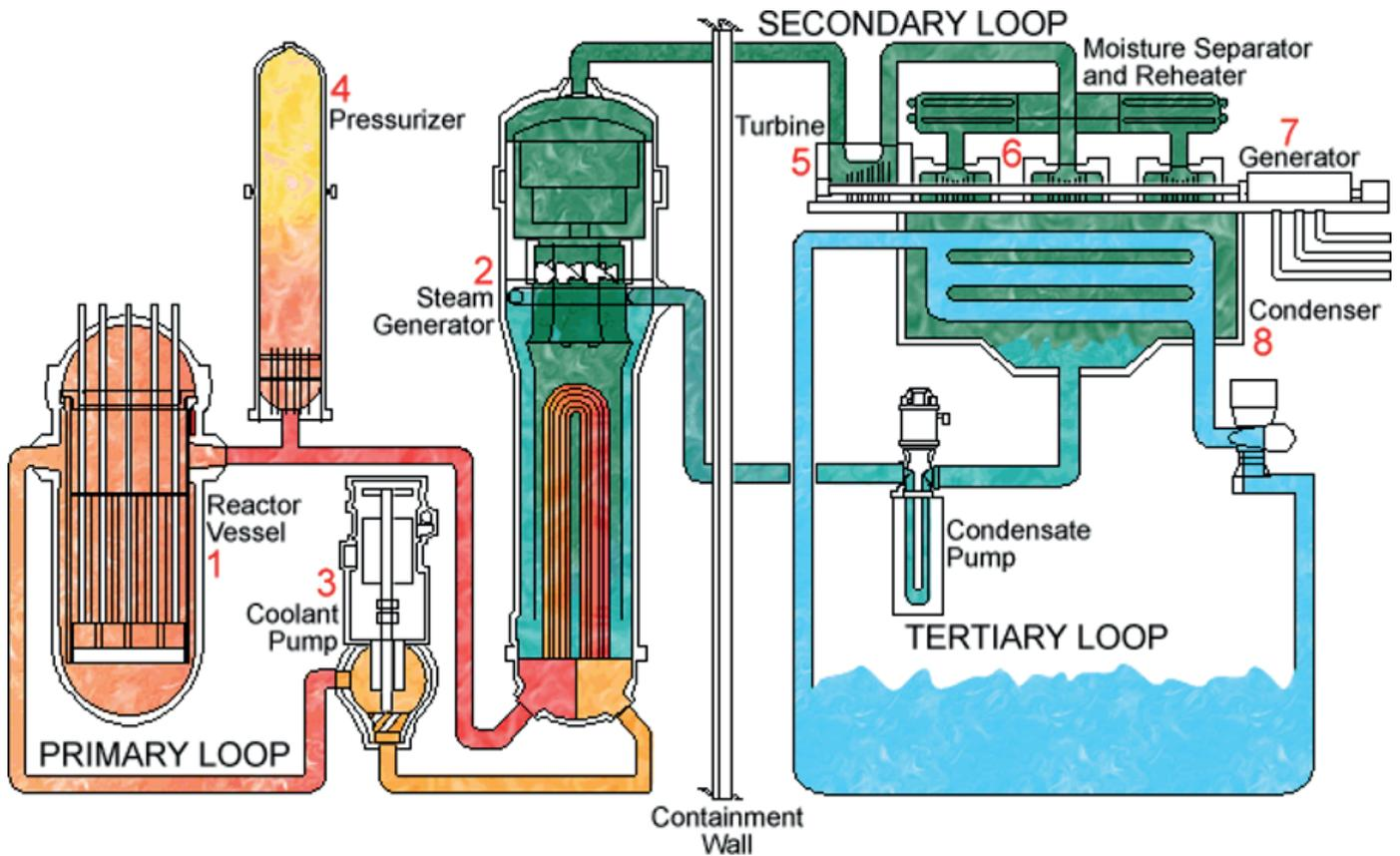
Koeberg operates on three separate water systems. The water is also known as the coolant. In other types of nuclear reactors, gas is used as the coolant. The fact that the three systems are separate is crucial because it means that the water in the reactor, which is radioactive but is in a closed system, does not come into contact with the other two systems and therefore does not contaminate the water in these systems.
