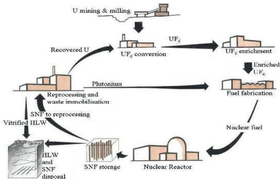
*A Typical Nuclear Fuel Cycle from Mine to Low-Level Disposal and Long Term Storage*
