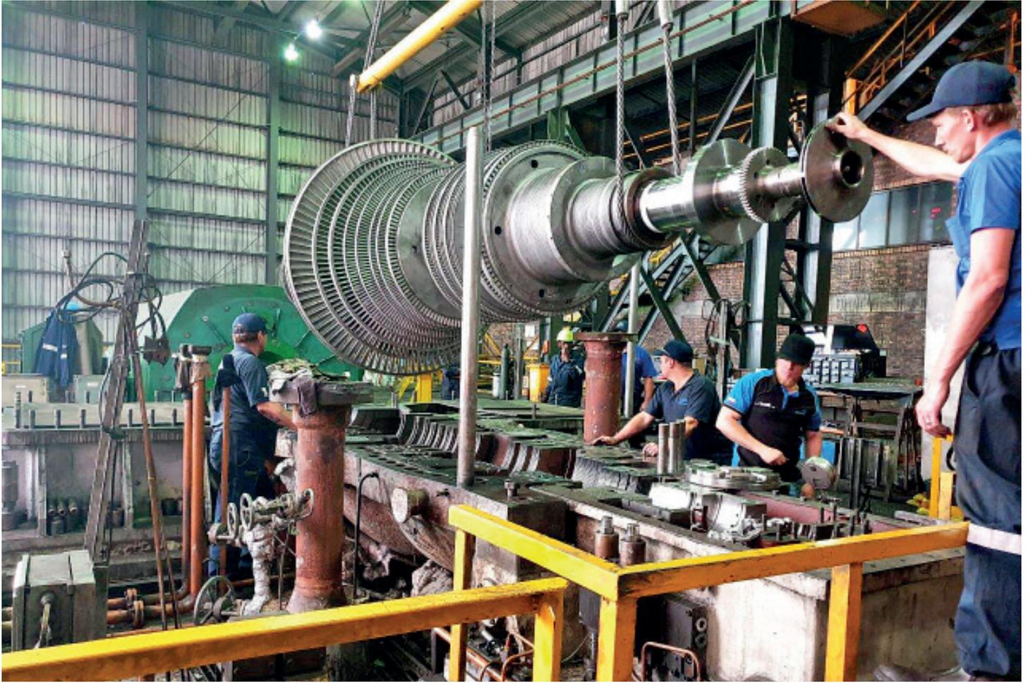
*ACTOM Turbo Machines technicians (from left) Louis Claasen, Jacques Zandberg and Dehan Meyer prepare to work on the 19 t rotor of the 40 MW turbine generator, as a rigger guides it into position.*
