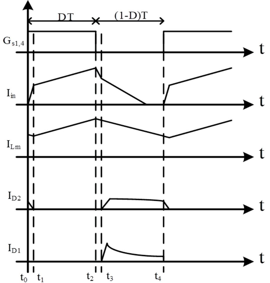
Figure 3: The proposed converter's equivalent waveforms in mode-I
