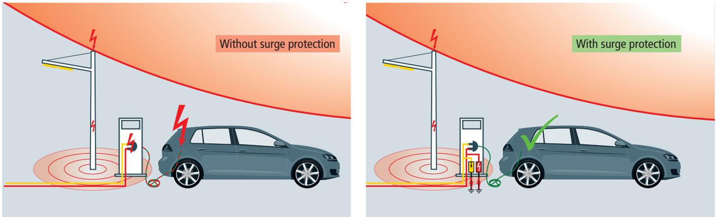
Figure 1 - Lightning and surge coupling when charging
