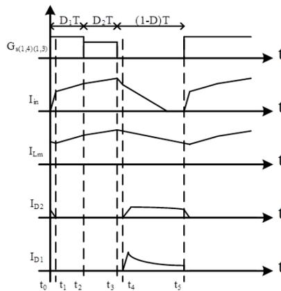
Figure 5: The proposed converter's equivalent waveforms in mode-II
