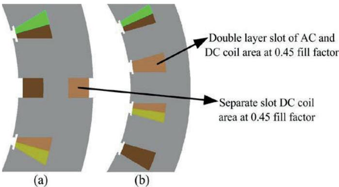
Figure 4: Depiction of the slot filling areas in 2D FEA modelling: (a) D-I, and (b) D-II.
