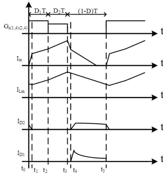
Figure 7: The proposed converter's equivalent waveforms in mode- III .
