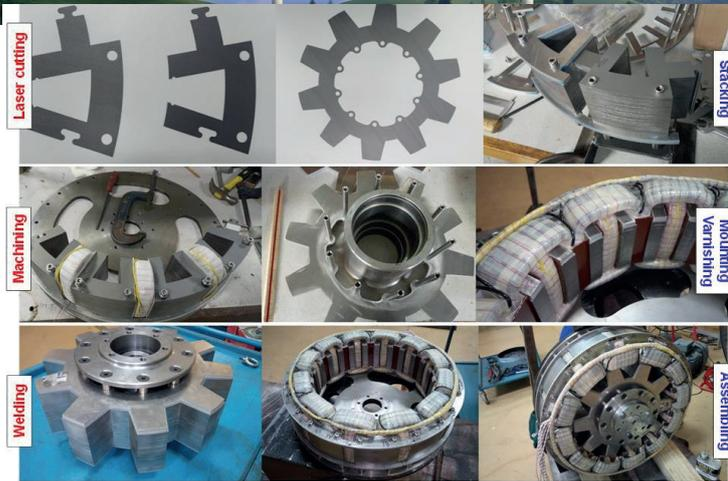
Figure 6: Manufacturing process of a 10 kW WF-FSM wind generator prototype<sup>15</sup>.
