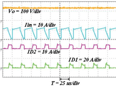
Figure 8: Experimental results for the proposed converter in mode-I.
