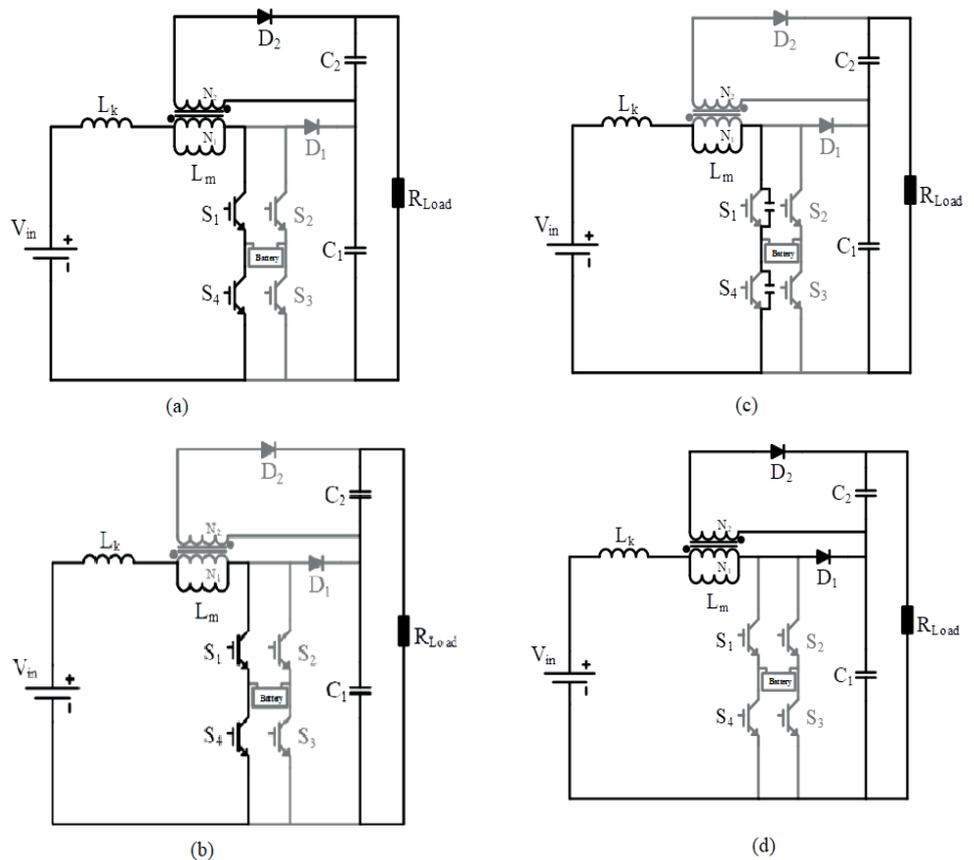
Figure 2: Sub-modes of the proposed converter in mode-I:
