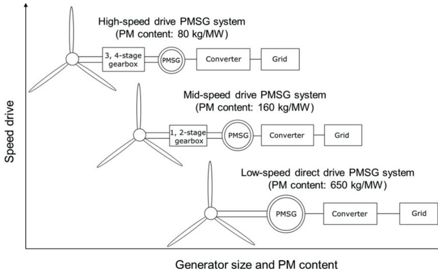
Figure 1: Wind turbines designed with PMSGs<sup>5</sup>.
