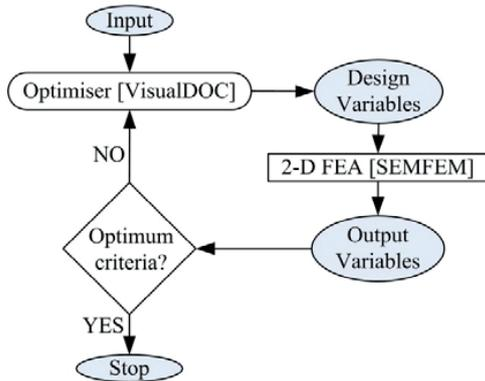
**Figure 3: An illustration of the design optimisation procedure.**
