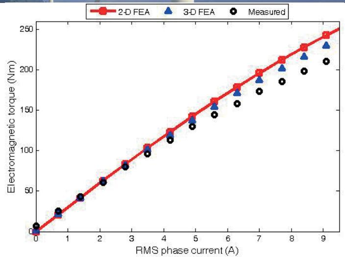
Figure 7: Measured electromagnetic torque under varying load current<sup>11</sup>.
