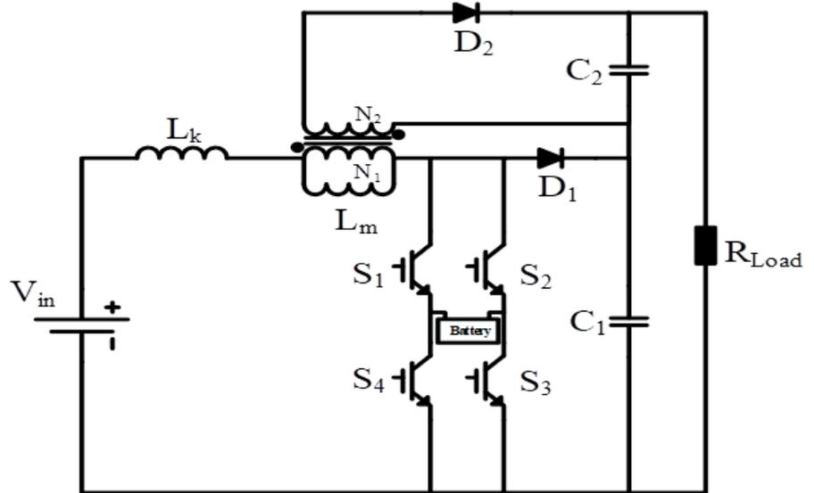
Figure 1: Circuit structure of the proposed converter.
