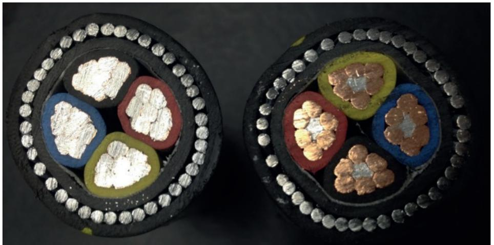
Example of low voltage utility cables with copper clad aluminium alloy (CCAA) conductors in accordance with NRS 110
