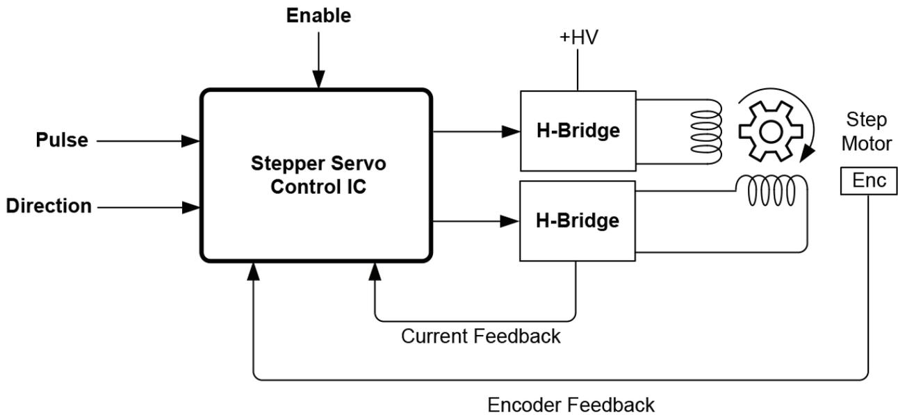
Figure 8: Stepper Servo Pulse and Direction Control
