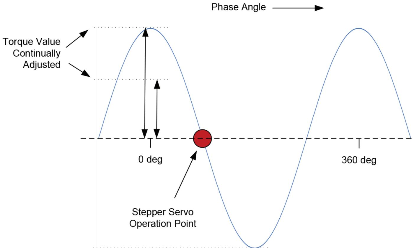
Figure 4: Stepper Servo Operation Point
