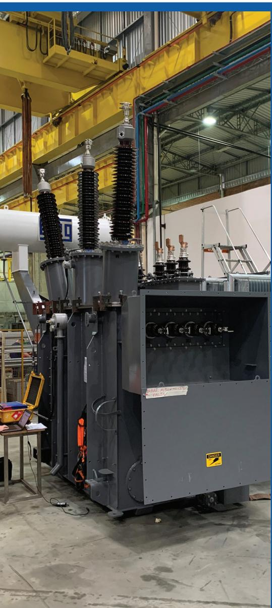
*Testing one of the WEG traction transformers during manufacturing*
