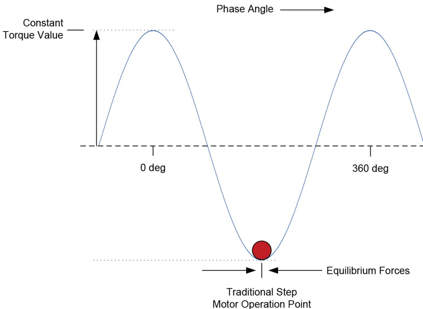
Figure 3: Traditional Step Motor Drive Scheme
