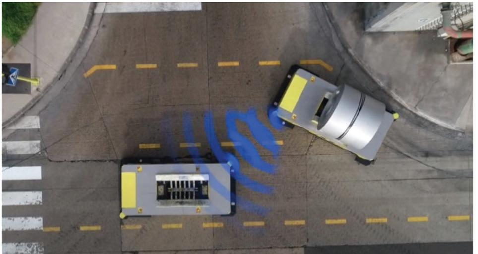
*A simulation of the AGV sensors guidance systems communicating with each other.*
