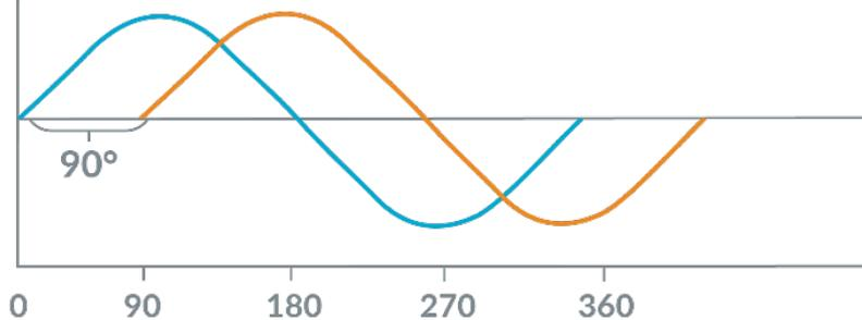
Figure 1: Traditional Step Motor Control Waveforms
