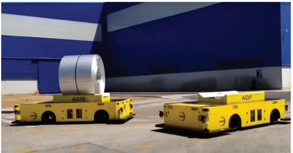
*The two AGV's in Acerinox Europa crossing at an intersection one with a 30 ton stainless steel coil payload.*
