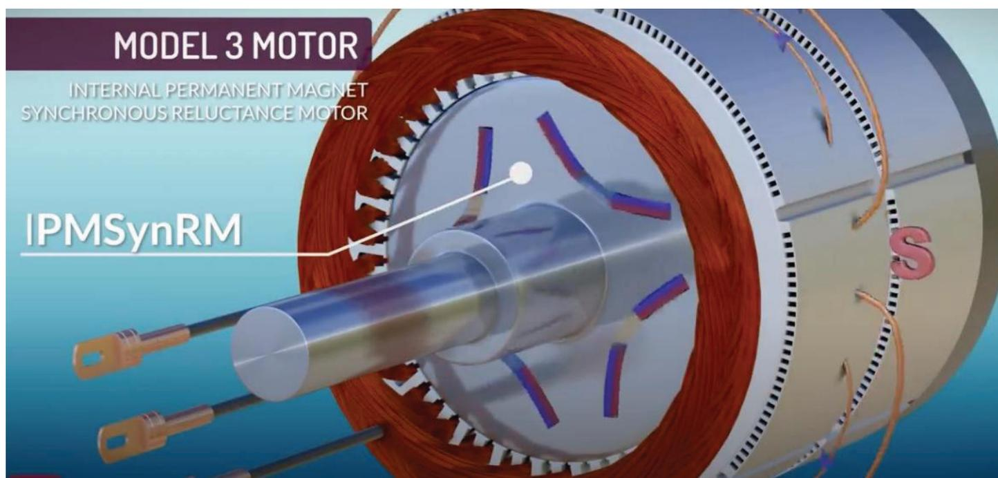
*Tesla vehicle reluctance motor with neodymium magnets embedded in the rotor*
