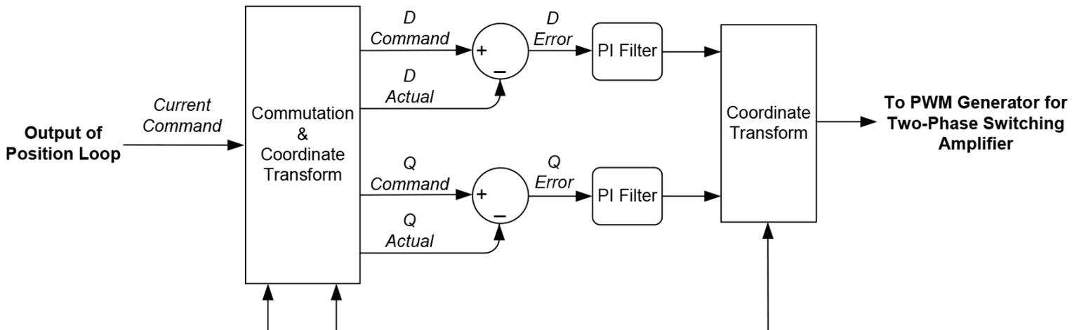
Figure 6: FOC Current Loop Diagram
