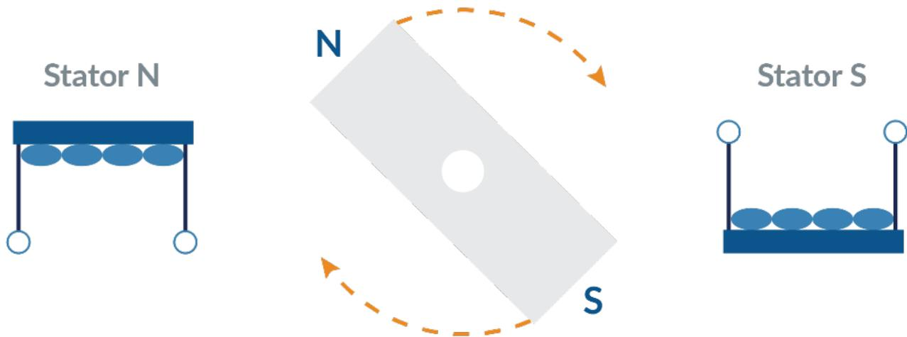
Figure 2: Spinning Bar Magnet Model for Step Motors
