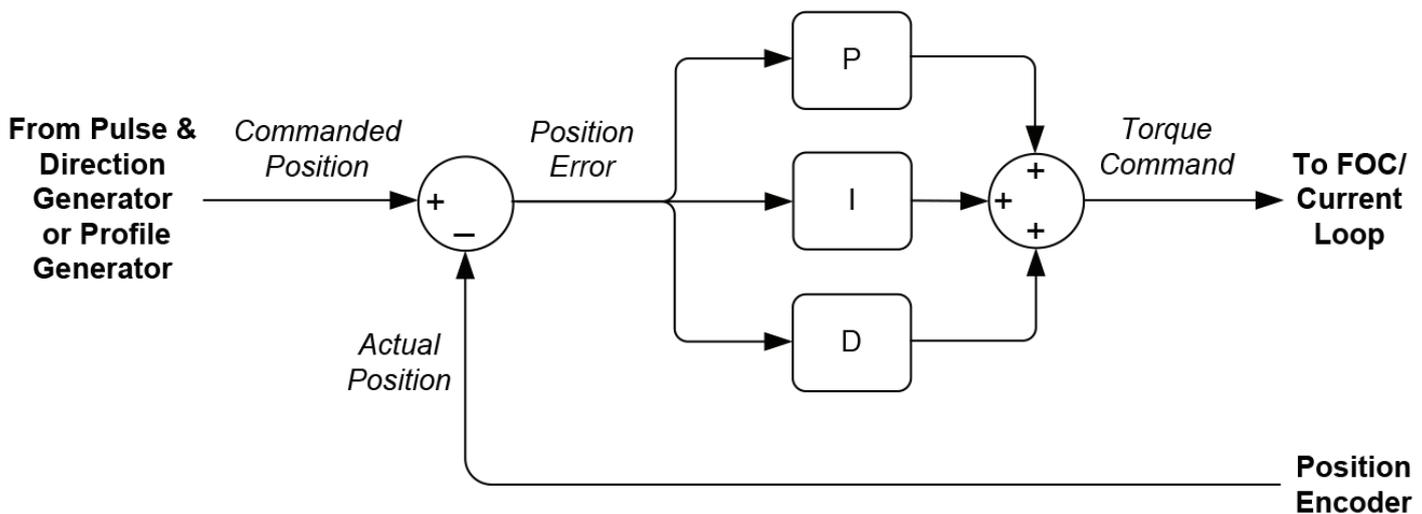
Figure 5: PID Control Loop
