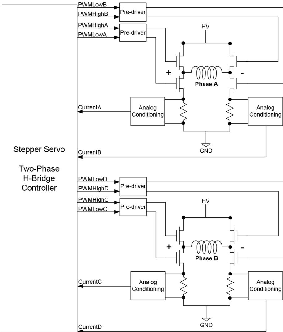
Figure 7: Bridge Control and Current Sense Scheme
