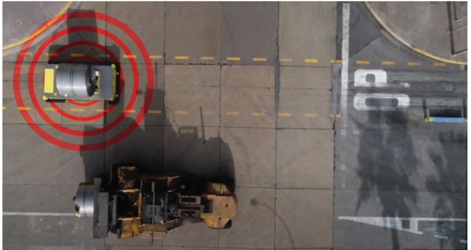
*Safety sensors continuously scan for obstacles. If detected the vehicle automatically stops.*
