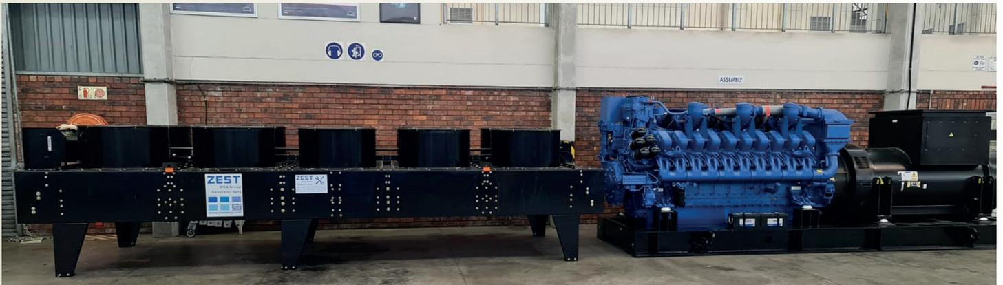
*Table top radiator with diesel engine coupled to WEG alternator.*
