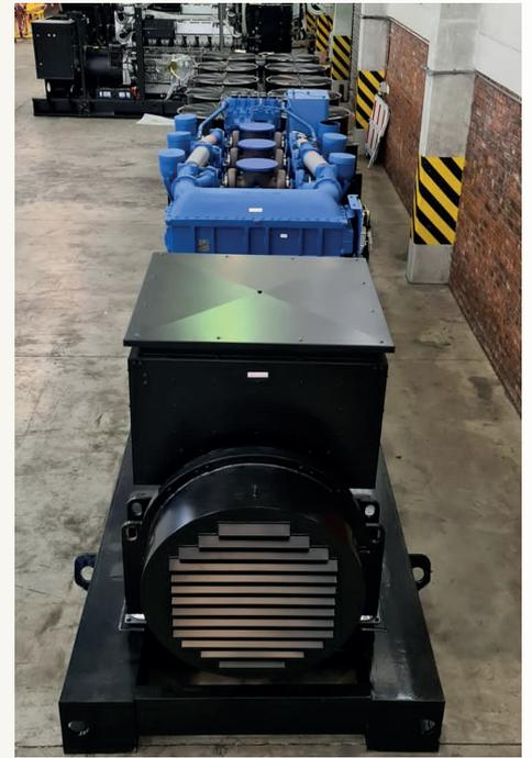
*The WEG MV alternator, in front, coupled to the diesel engine.*
