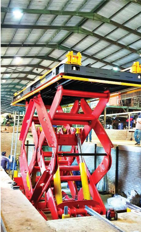
Up and coming dock-levelling manufacturer, REV Designs, recently completed the design and construction of three of the country's largest scissor lifts ever produced with a capacity of up to 40 tons per lift.
