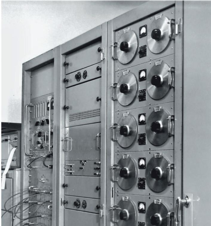
Figure 18: Ultimately 50 oscillators of this design were constructed by the SA Post Office.
