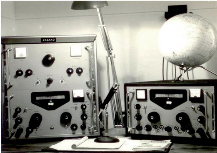
Figure 20: Gijs de Vries also constructed an exciter (L) in the genre of the Racal MA79 and a linear amplifier (top) to match the RA17 clone he constructed (R).
