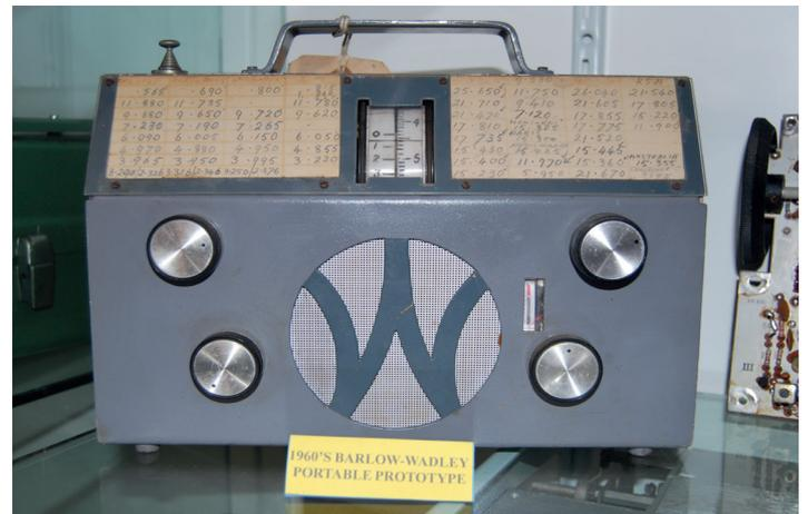
Figure 21: Wadley transistorised portable prototype.
