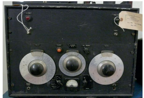
Figure 19: Cascaded Wadley heterodyne wavemeter and oscillator (note the front panel meters to monitor key voltages and currents like the prototype receivers)
