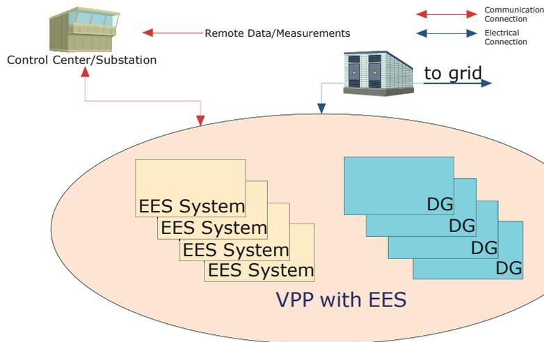
**Figure 3-19 | A generalized control concept for aggregated EES systems and DGs (ABB)**
