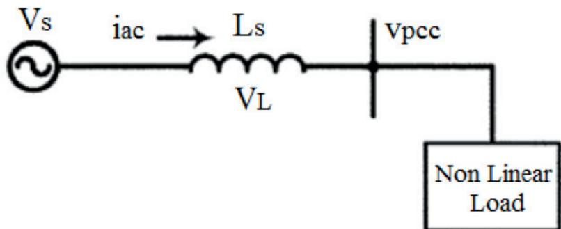
load currents. Thus, in principle, end users and utilities share responsibility for limiting harmonic current injections and voltage distortion at PCC. Since there are two parties involved in limiting harmonic distortions, evaluation of harmonic distortion is divided into two parts: measurements of the currents being injected by load and calculations of frequency response of system impedance.
