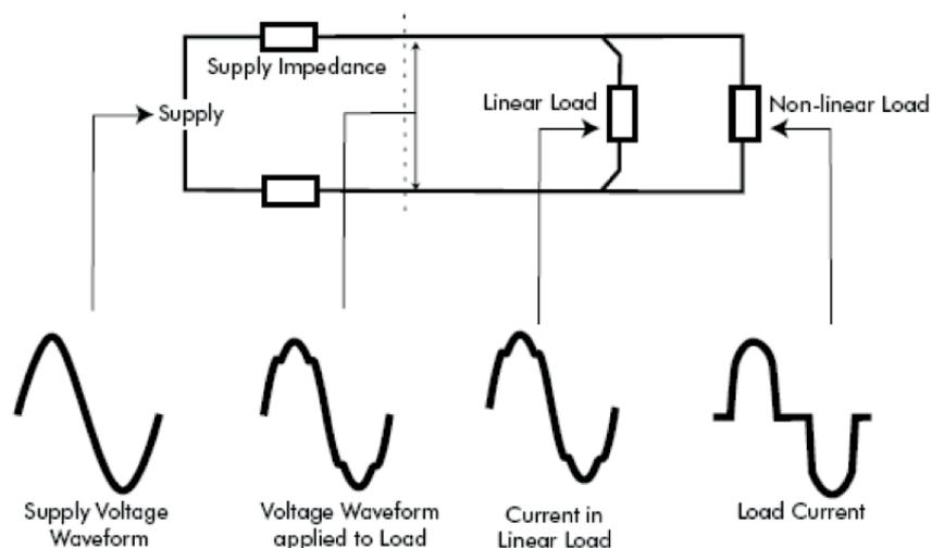
Voltage Distortion - Close Coupling
