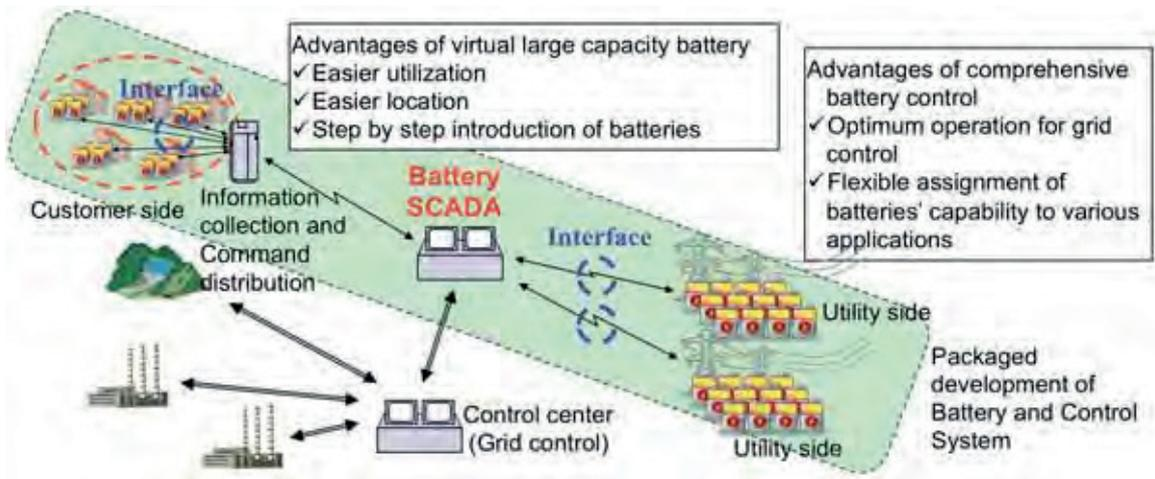
**Figure 3-20 | Schematic diagram of Battery SCADA (TEPCO)**
