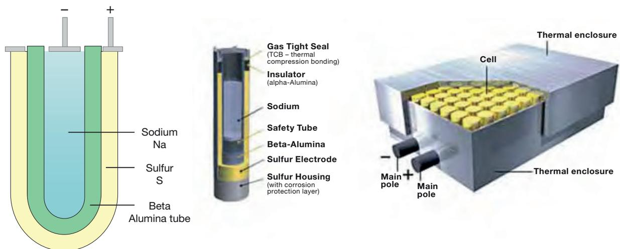
Figure 2-6 | NaS Battery: Cell design and 50 kW module (NGK, IEC MSB/EES Workshop 2011)
