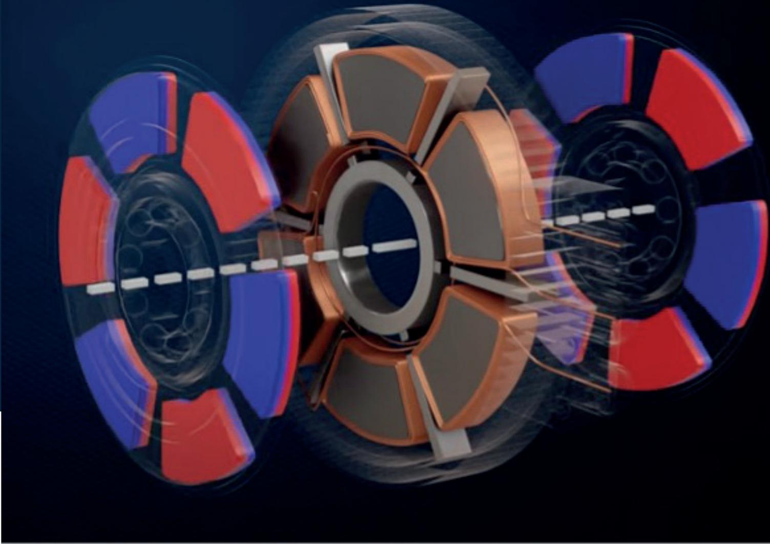
*Axial flux motor components - The rotors with permanent magnets will usually be fixed to the shaft, and the stator with windings fixed to the housing. The hinted ball bearings in this illustration indicate a direct drive vehicle motor with rotating housing and power supply through the stationary shaft.*
