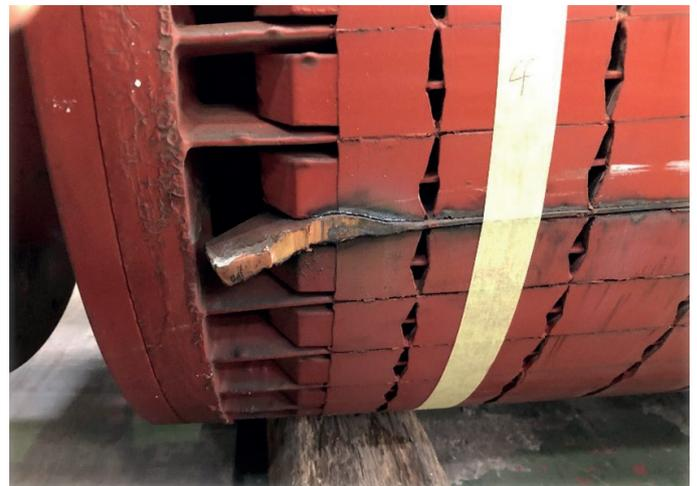
10. Rotor bar fractured and lifted damaging the stator winding.
