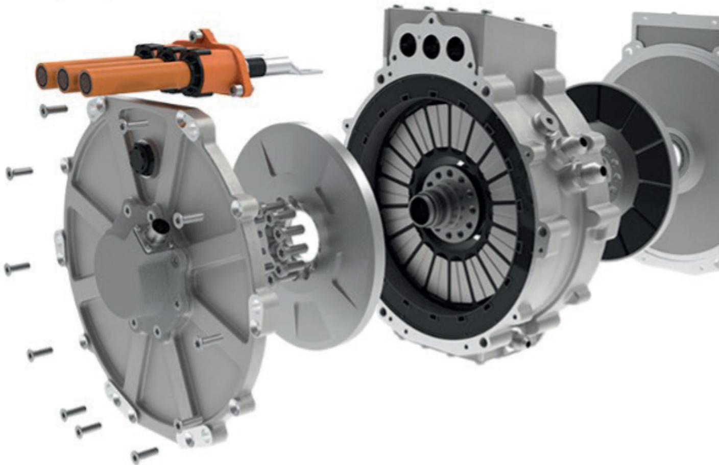
*Exploded view of an axial flux motor showing 18 electromagnet stator cores mounted in housing and two permanent magnet carrying rotors which can be bolted to the shaft. Note the 3-phase connecting box at top of housing and cooling air connections at side.*
