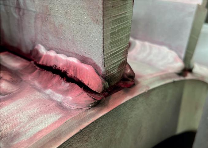
7. Aluminium Bar welding Failure.
