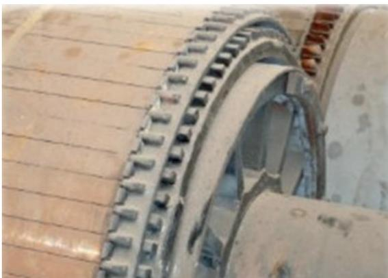
3. Double Cage Bar Wound Motor Rotor.
