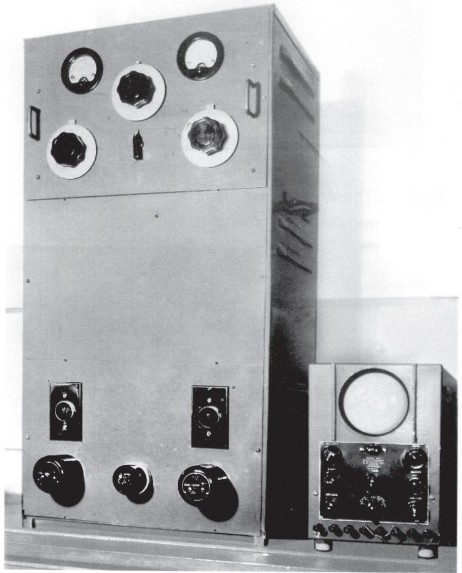
Figure 7: G.D. Walker's ionosonde that observed the effects of the solar eclipse in 1940.
