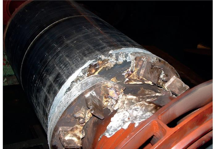
8. Cast Aluminium Rotor Failure.
