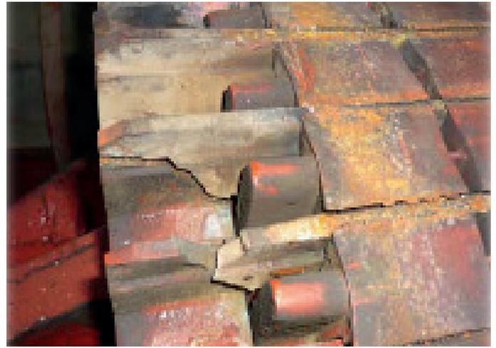
6. Cage Bar Wound Induction Motor Rotor Failure.
