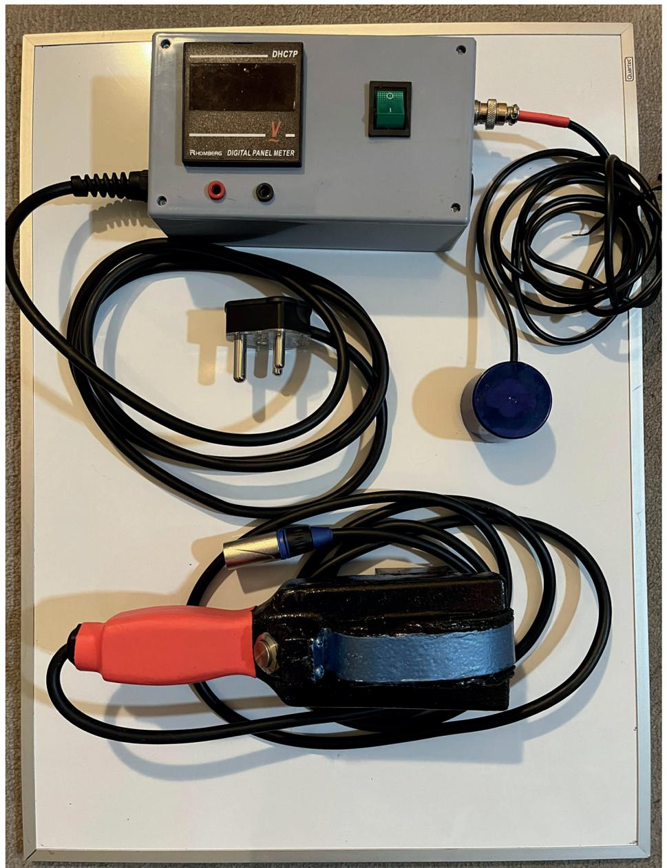
*Growler with Power Supply, Voltmeter and Pick-up Coil.*
