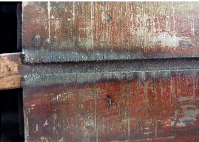
9. Rotor Lamination Core burning due to fracture bar.
