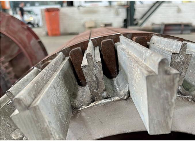
5. Aluminium Rotor bars brassed to Aluminium end rings.
