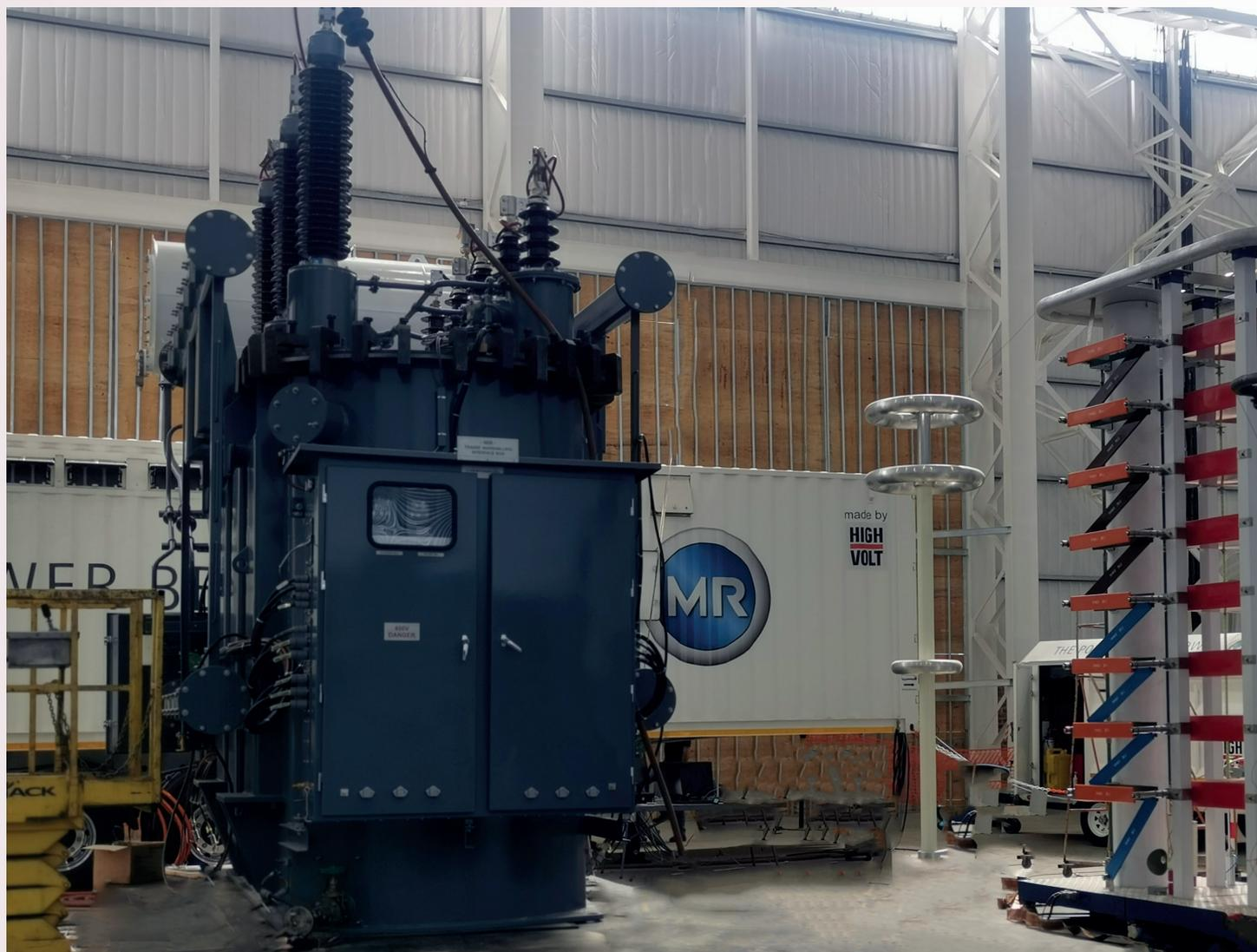
SGB-SMIT POWER MATLA is proud to celebrate a significant milestone marking the commissioning and operation of the on-site testing facility since the fire accident at the Pretoria power manufacturing plant in March 2021. In the newly built on-site test facility, the team successfully manufactured and tested a 45MVA 88/11kV double-wound three-phase transformer manufactured for a local utility on 8 March 2022.
