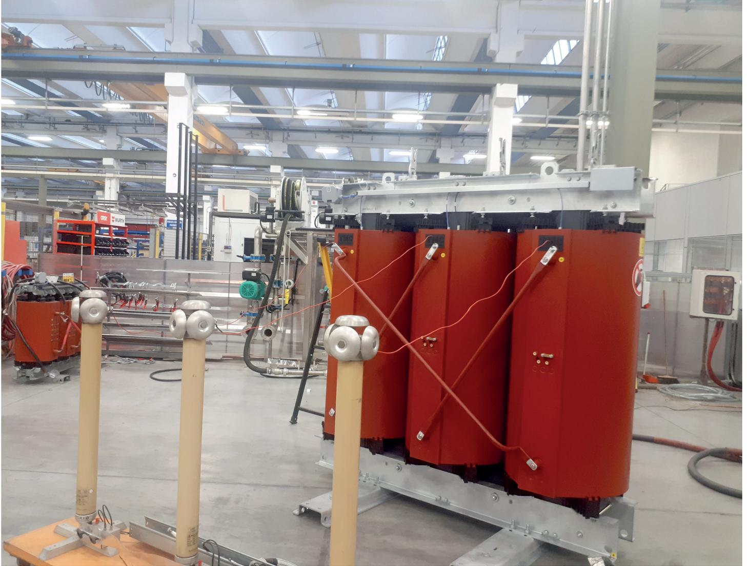
*Measurement of partial discharge level during routine testing.*
