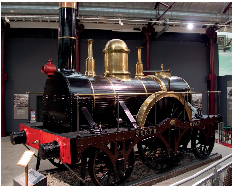
A 2-2-2 locomotive "North Star" with 7-foot driving wheels used from 1837 to 1871.
