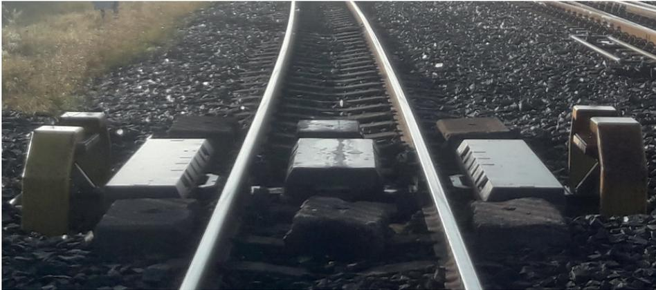
*Wheel profile measuring equipment at Ermelo (Source: S. Tosen)*
