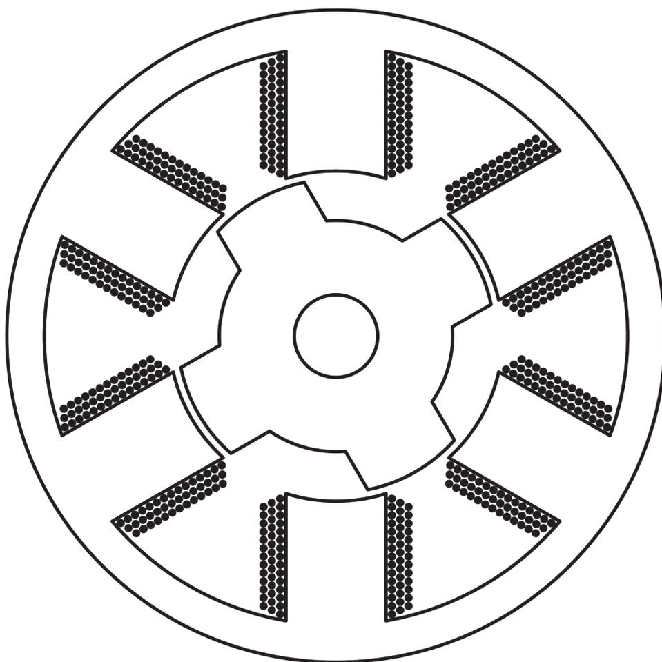
*Cross-section of switched reluctance machine with 6 stator and 4 rotor poles. Notice the concentrated windings on the stator poles.*
