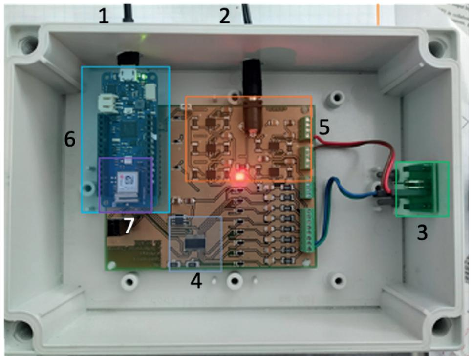
Figure 4. The physical implementation of the magnetostrictive sensor circuit.
