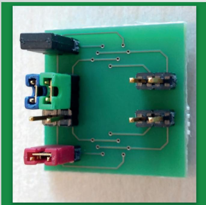
(c) Picture of the lower side with jumper inserted.
