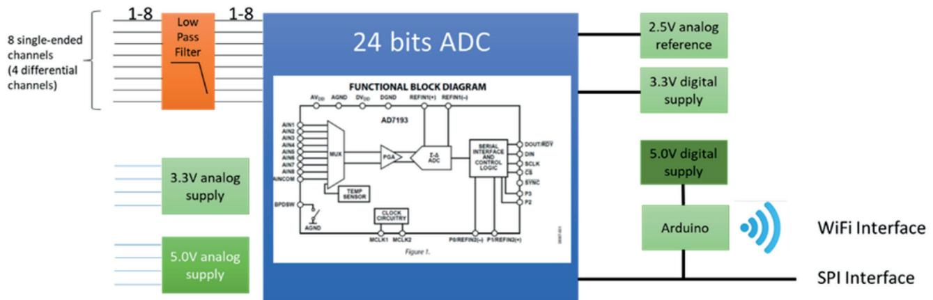
Figure 3. Block diagram of the magnetostrictive sensor circuit.
