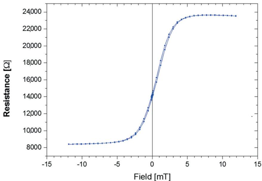
Figure 1. Measured resistance variation of the magnetic tunnel junction (MTJ) sensor with a magnetic field.
