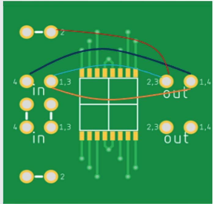
(b) PCB testing connections for one bridge.
