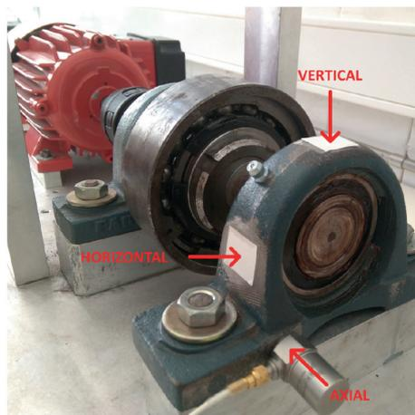
Figure 5. Motor load with 3 locations for fixing the accelerometer for vertical, horizontal and axial measurements.
