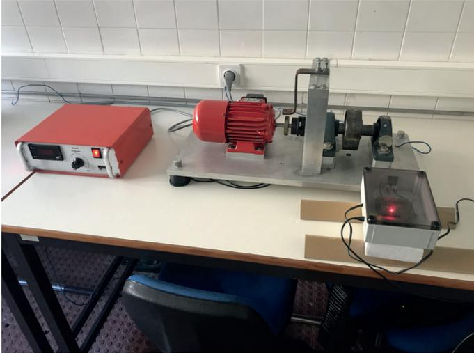
(a) Setup for the vibration measurements on the horizontal axis.
