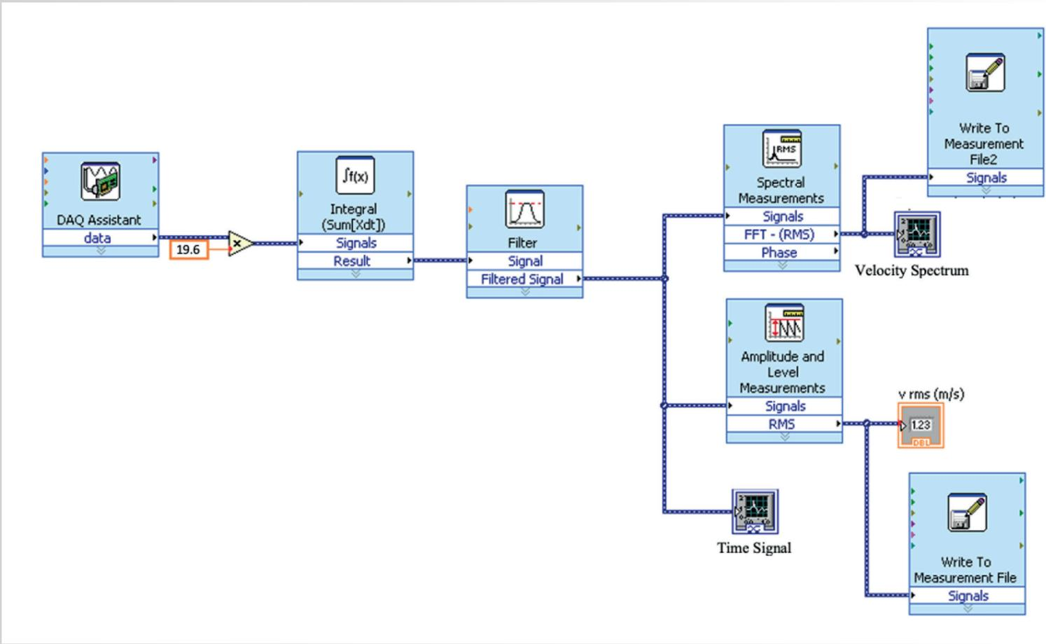
Figure 6. Extract of the software program, developed in LabView, for acquisition, processing, visualisation, and signal storage.
