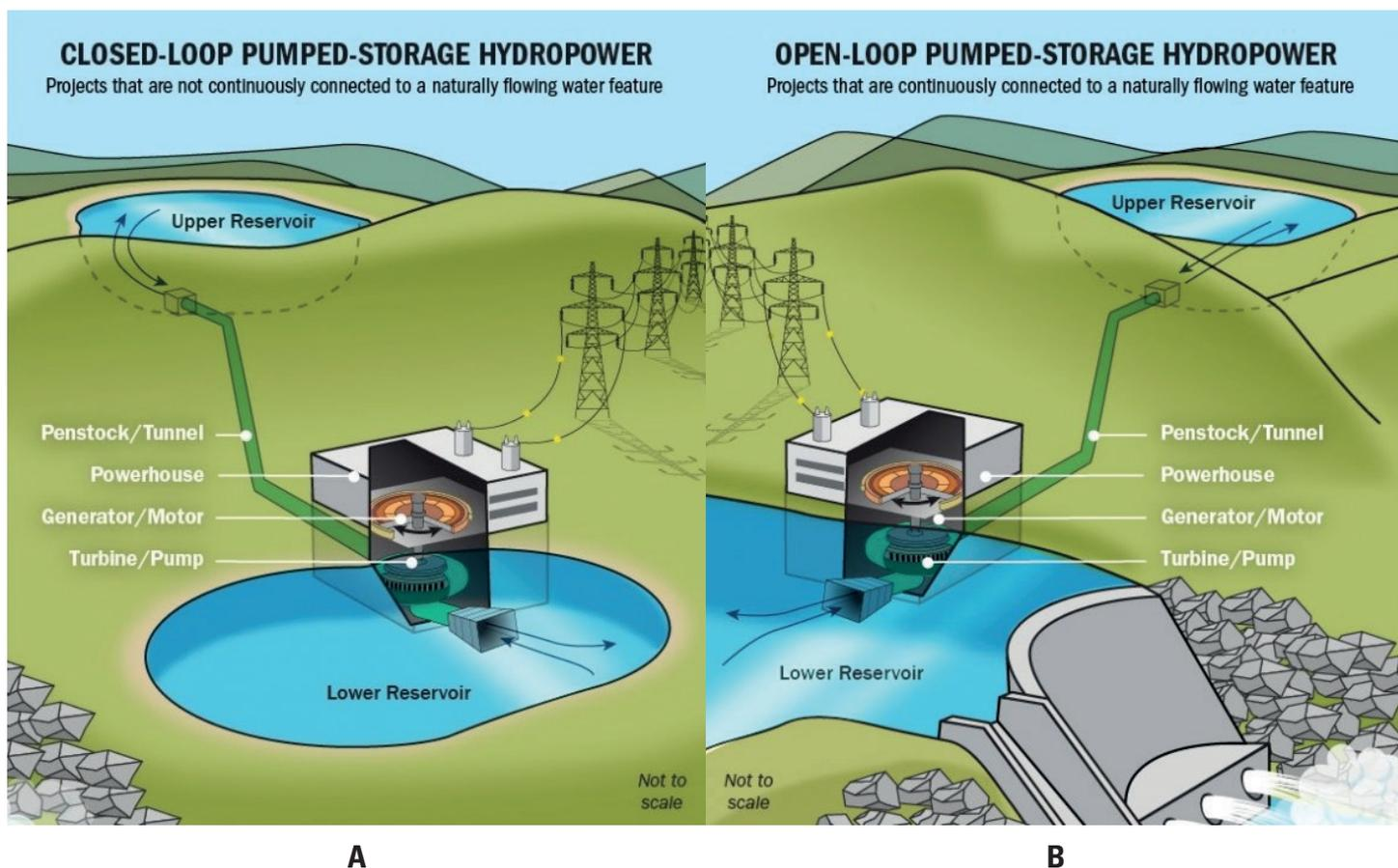
Figure 7: Pumped storage facility structures.
