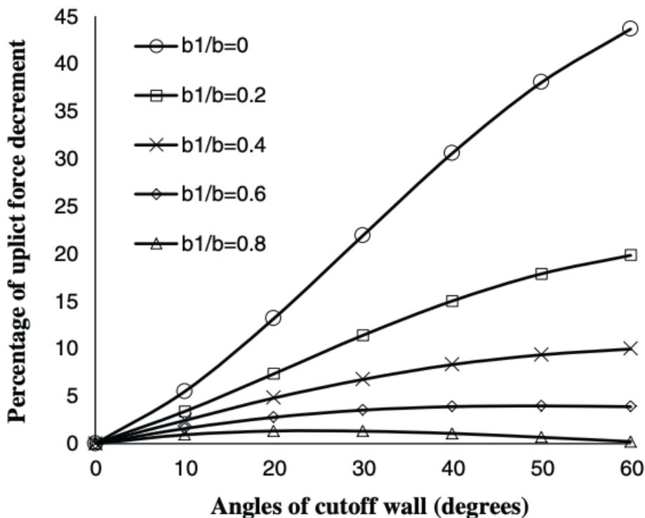
Figure 5: (a) Comparing the effects of the location and the angle of the cut-off wall for uplift force. (b) Comparing total uplift force on the different angles of the cut-off wall to the right-angled condition [7].
