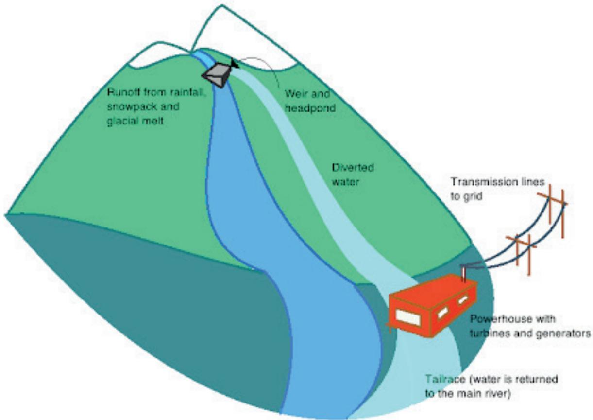
Figure 4: Diversion facility structure [6].
