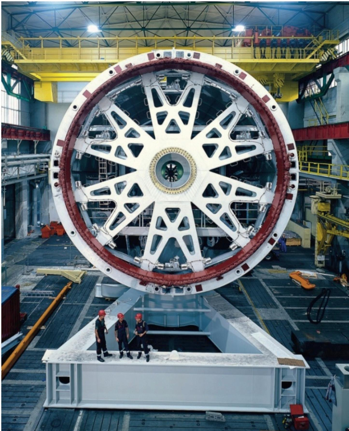
*A direct drive permanent magnet turbine alternator*
