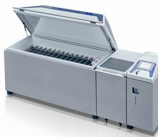
A precision two-component nozzle ensures optimal spray mist distribution. The two material nozzles are used to nebulise the salt solution in the testing chamber. These are arranged in specialised spraying channels in the walls of the chambers.
