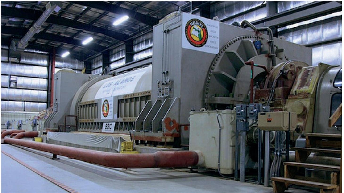
*The 1,2 GW motor generator system which powers the outer coils on the LANL 100 T pulsed magnet.*
