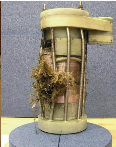
*The LANL 80 tesla pulsed test magnet before and after 10 pulses*
