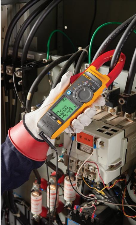
*The Fluke 377 FC and 378 FC True-rms clamp meters use Field-Sense™ technology to make testing faster and safer, all without touching a live conductor for accurate voltage and current measurements.*
