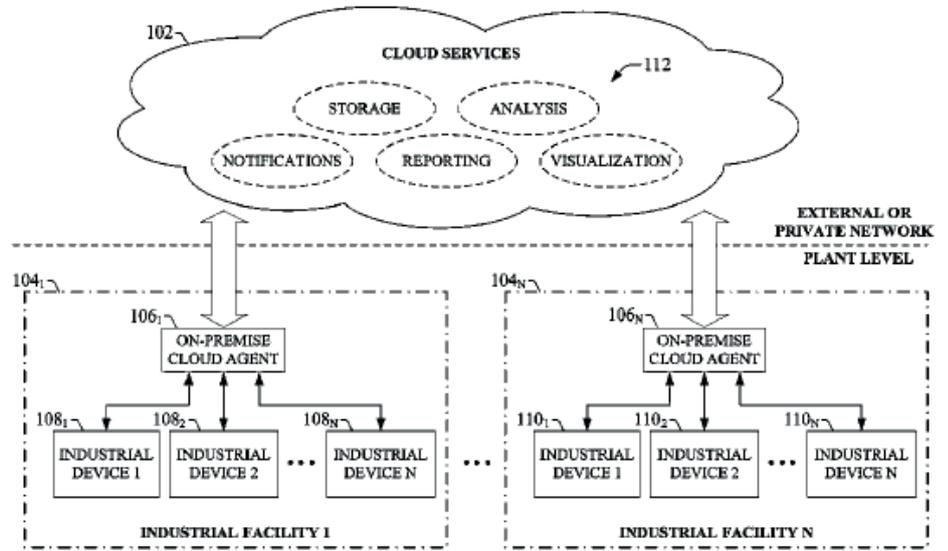
Figure 1: Remote Monitoring system [3]
