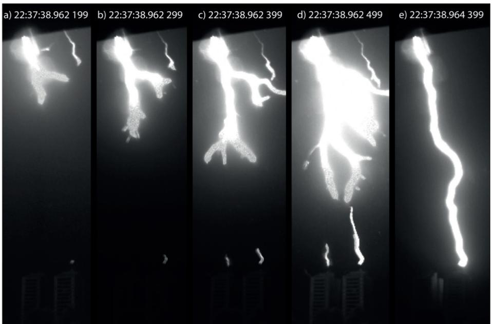
Figure 1: A sequence of frames from one of the high-speed captures of a lightning attachment to the apartment building on the left. The downward leader propagation can be seen as can two upward leaders - an upward unconnected leader (left) and the upward connecting leader (right) [2].
