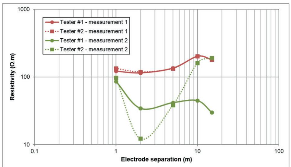
Fig 2: Example of discrepancy in soil resistivity measurement
