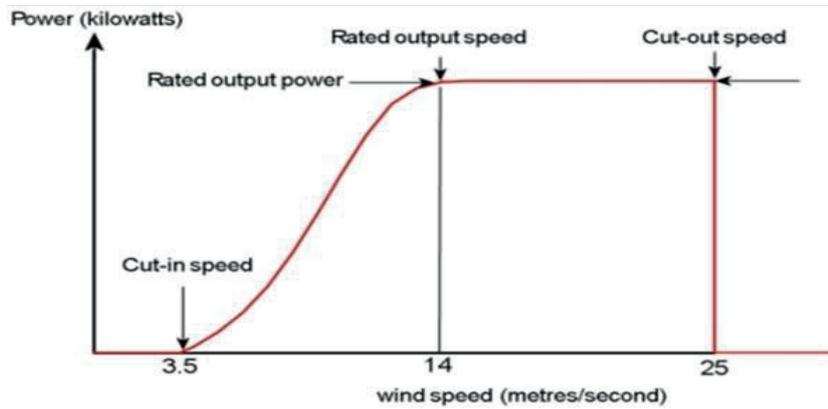
Figure 4: Power generated with respect to speed for WES [11]
