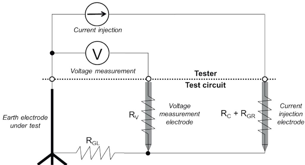
Fig 6: More accurate "earth resistance" laboratory test principle (three-wire internally connected method as an example)
