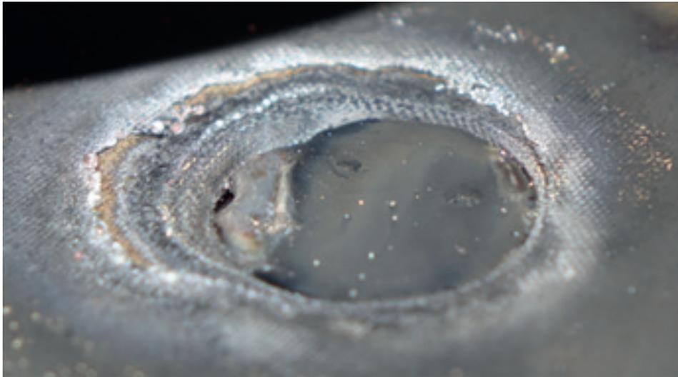
Figure 6: Damage to receptor outside of charge limits
