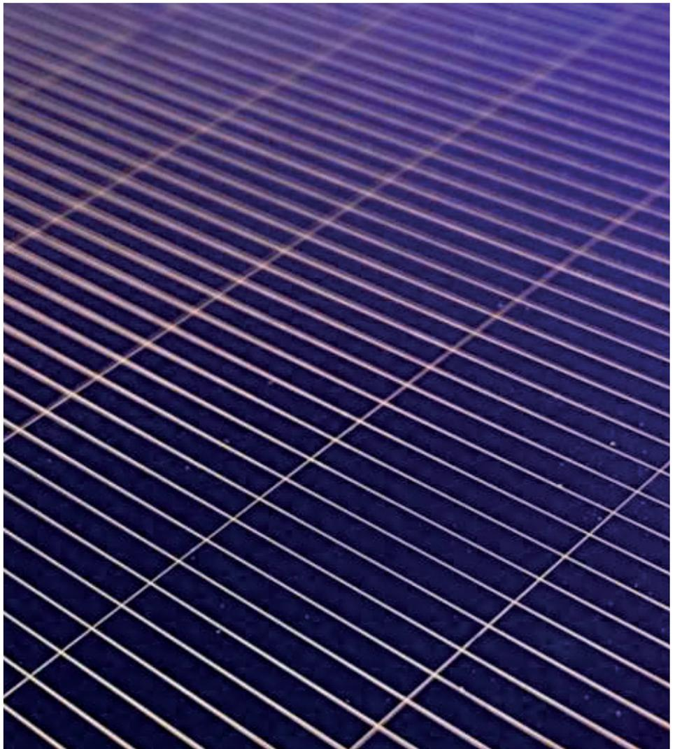
*At just 19 micrometers in width, the copper contacts are extremely thin. As a result, the light-sensitive silicon layer does not experience much shading. Credit: PV2+*
