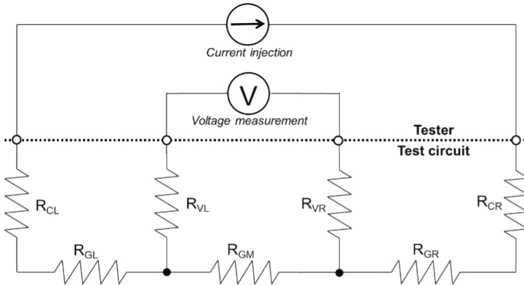
Fig 3: "Soil resistivity" laboratory test circuit
