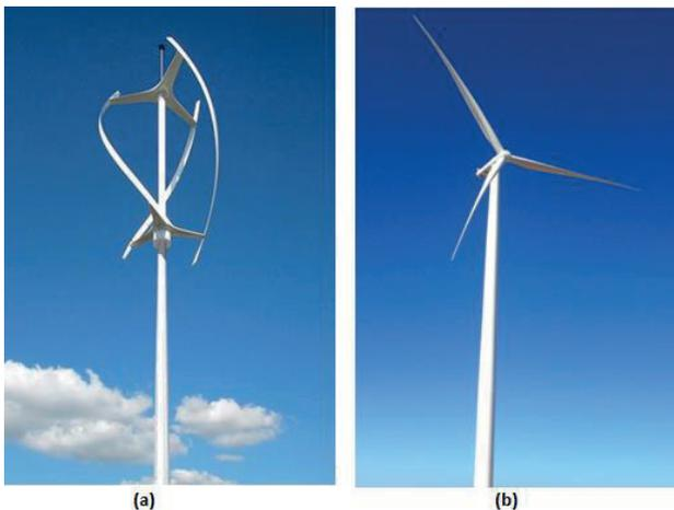
Figure 3 (a) Vertical Axis Wind energy system turbine [4]; (b) Horizontal Axis Wind energy system turbine [8]
