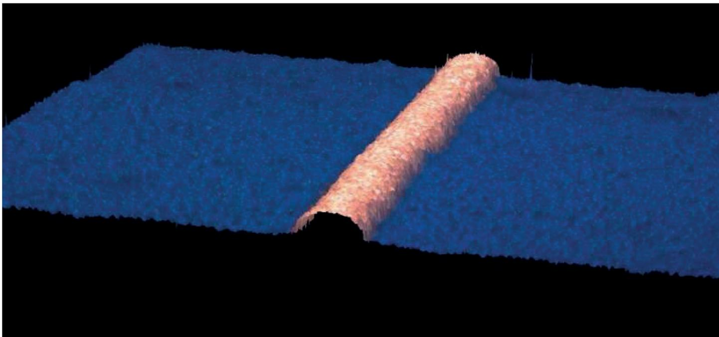
*Three-dimensional confocal microscopy image of a copper contact produced using the laser-assisted process developed by PV2+. The contact's exact, semi-circular shape ensures a high electrical conductivity level. Credit: PV2+*
