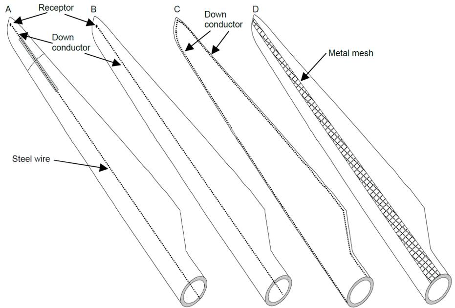
Figure 4: Lightning protection concepts for modern wind turbines
