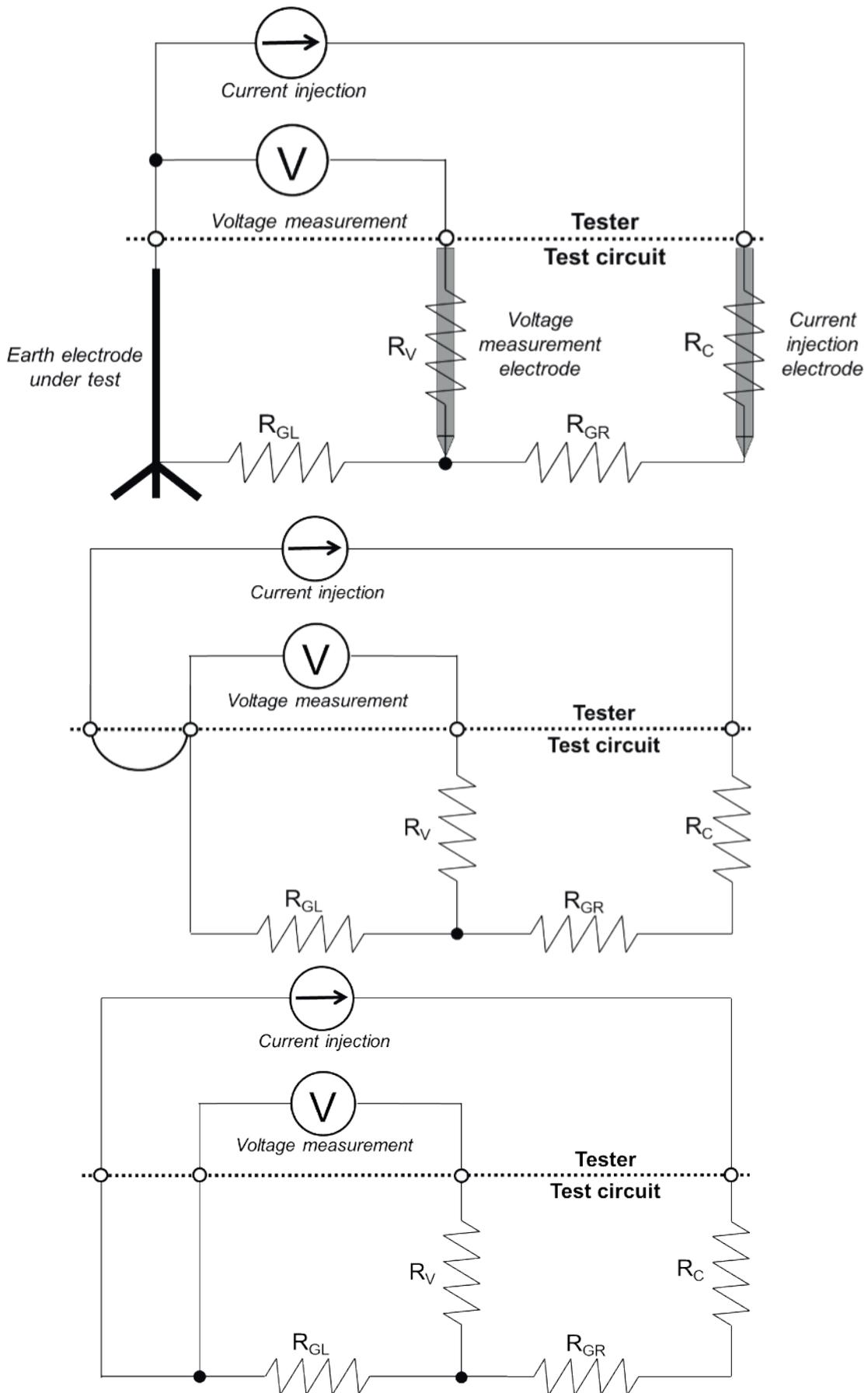
Fig 5: Laboratory "earth electrode" resistance test principle - 3-wire internally connected (above), 3-wire external connection (centre), 4-wire connection (below)
