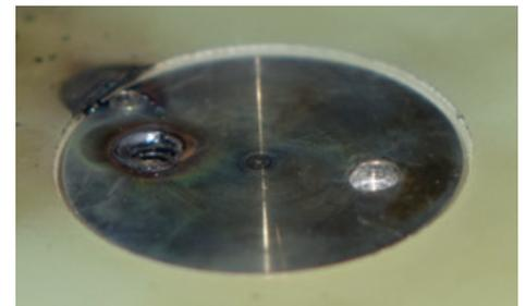
Figure 5: Damage to receptor within charge limits (20c)
