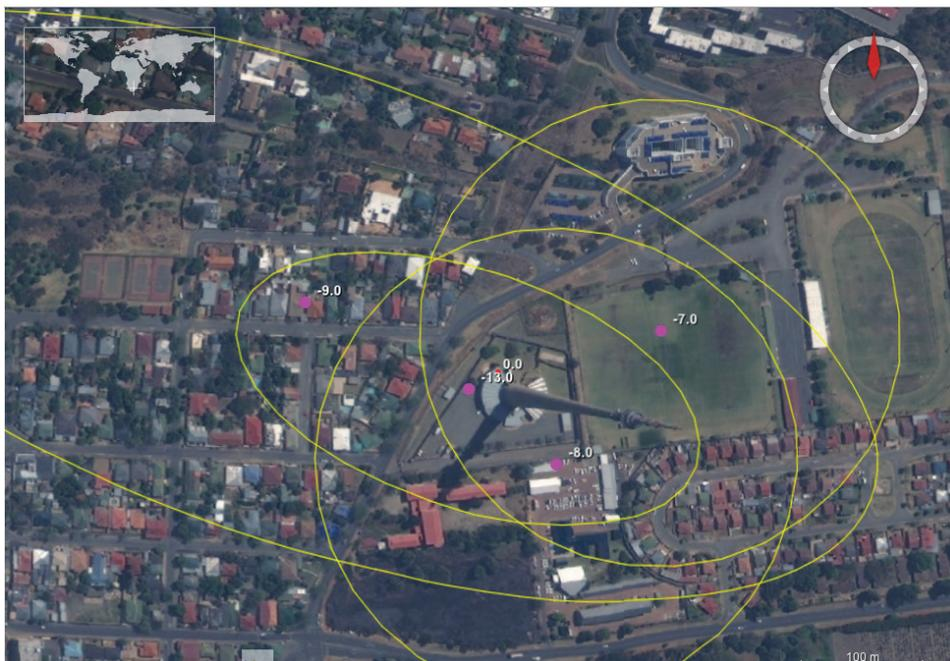
Fig 4: SALDN LLS CG flash report - 4 detected strokes - reported locations not on tower
