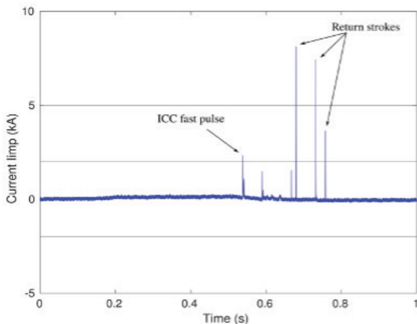
Figure 5: A typical upward lightning current waveform measured at Sentech tower during the 2020 to 2021 thunderstorm season.
