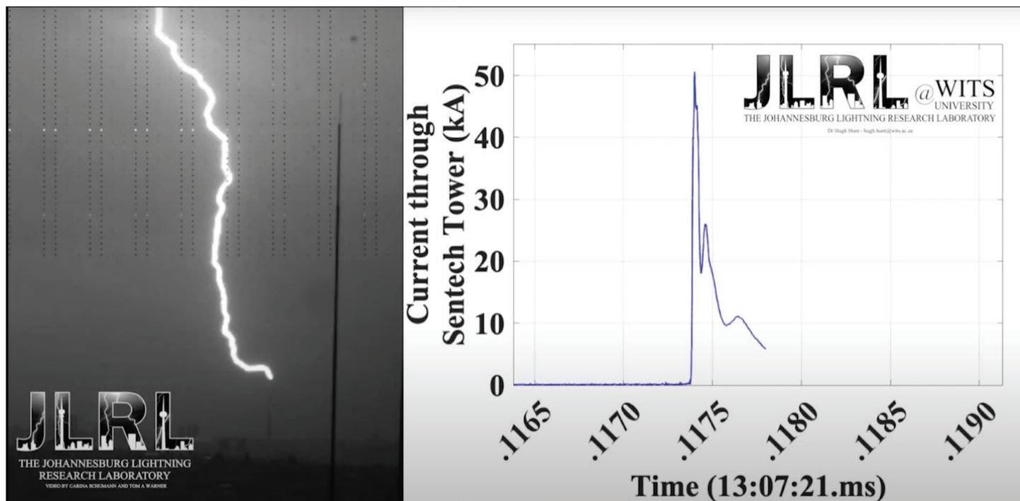
Figure 4: The first lightning current measurement made at the Sentech tower on 5 October 2020 at 13:07:21 UTC. A rare case of a downward lightning event to the tower. The full clip can be viewed [here](#).
