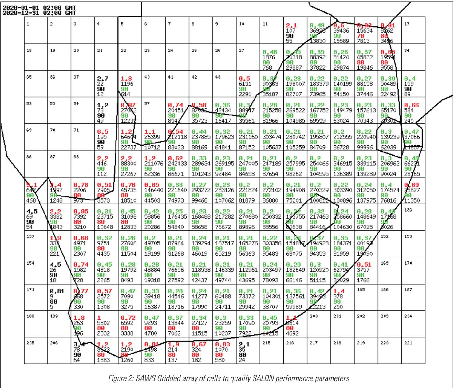
Figure 2: SAWS Gridded array of cells to qualify SALDN performance parameters
