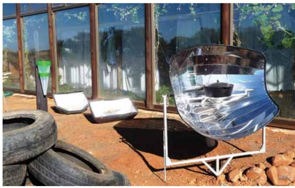
Fig 7. Let the sun do the work with two solar stoves and the 1kW solar oven.
