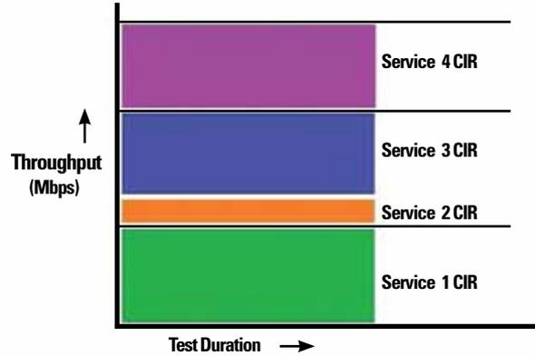
Figure 3: The Performance Test of Y.1564 verifies that the maximum throughput (CIR) of each service can run simultaneously.
