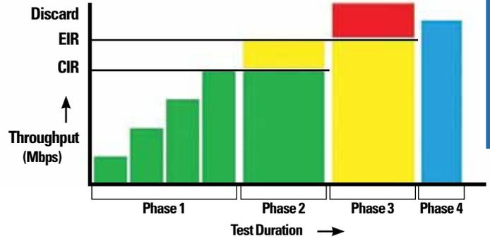
Figure 2: The four phases of the Y.1564 Configuration Test. The duration of each phase is user defined.
