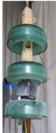
Figure 13: Insulator and prototype's enclosure covered with dried saltwater
