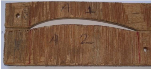
Fig. 2: Plywood template for Rutland timber blade construction
