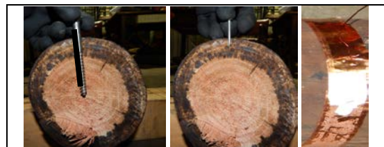
Figure 5: Partially insulated coach screw penetration (left), nail penetration (centre), copper strap (strap)
