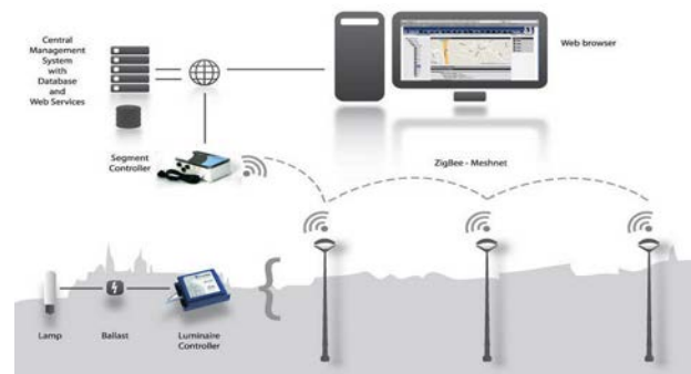
Figure 1: Typical Street Light Management System [6]
