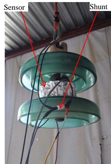
Figure 7: Position of leakage current prototype and shunt resistor
