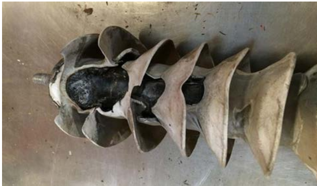
Figure 6a: SA where the housing has been punctured
