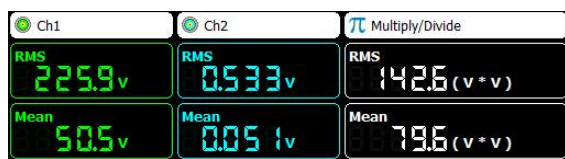
Figure 14: Captured RMS current and voltage input of 220V AC supply
