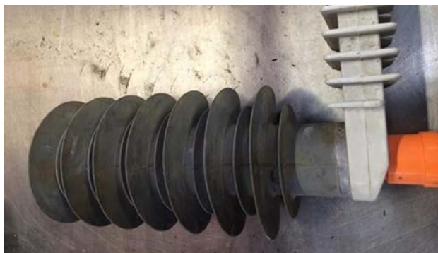
Figure 6b: SA where the housing is intact
