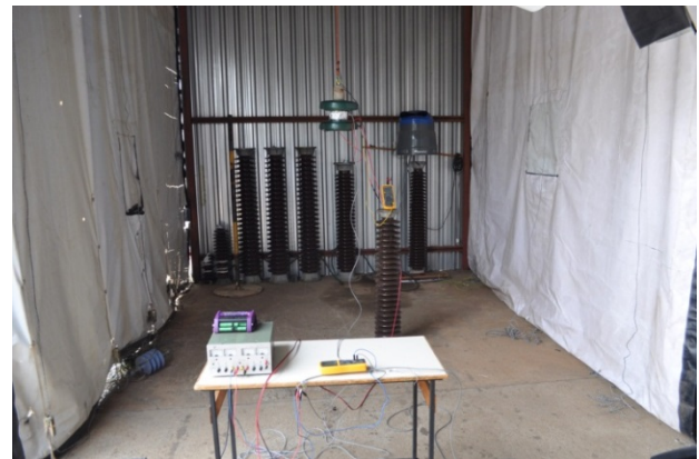
Figure 6: Calibration test setup for the leakage current prototype and the shunt resistor
