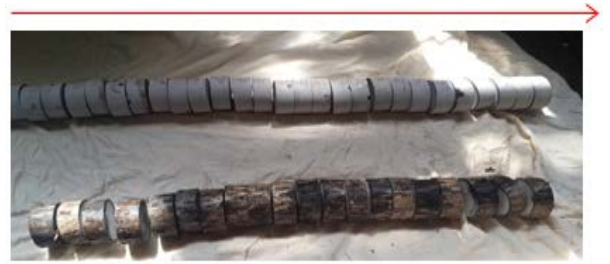
Fig 9: Varistor blocks that were tested.
