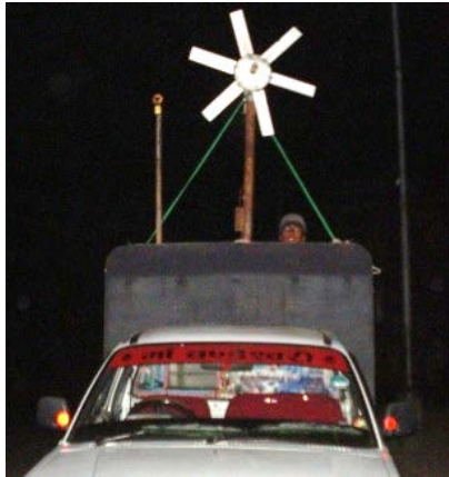
Fig. 4: Rutland wind turbine system under test on vehicle
