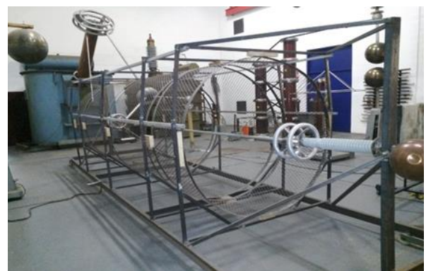
Figure 3: The full corona cage under test
