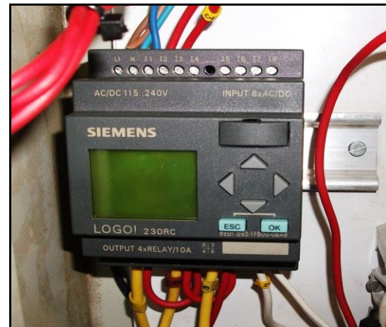
Figure 5 Siemens PLC integrated with the control system
