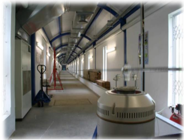
Fig 1. Test span length 85m, at University of KwaZulu-Natal (UKZN) Vibration Research and Testing Centre
