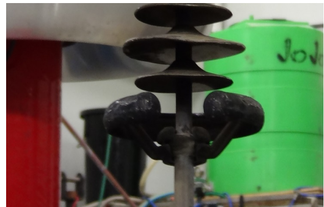
Figure 4: Burnt grading ring
