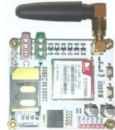
Figure 2. GSM module with attached antenna and MTN sim card
