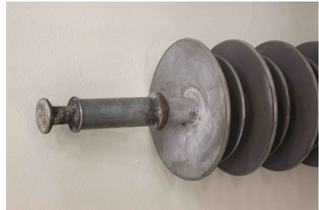
Figure 3: Longrod polymer insulator end fitting damage
