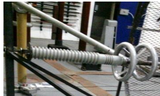
Figure 2: Corona rings at the end of the test conductor
