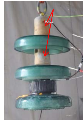
Figure 10: Leakage current test setup using two stand-off glass insulators
