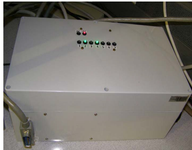
Fig. 4: Programmable GPIB switching isolator (up to 7 channels)
