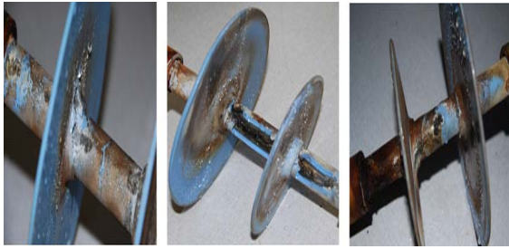
Figure 8: Hydrophobicity assessment for the insulators aged with HVAC, positive polarity HVDC and negative polarity HVDC respectively.
