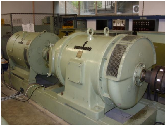
Figure 1: The 520kVA generating set in the machines laboratory of the University of Cape Town
