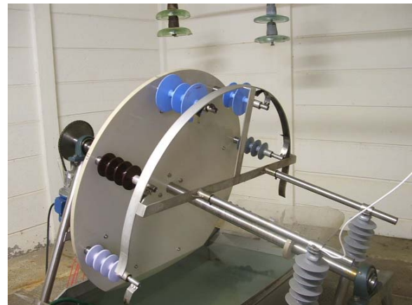
Figure 1: The Tracking Wheel Tester showing six samples tested simultaneously [4].
