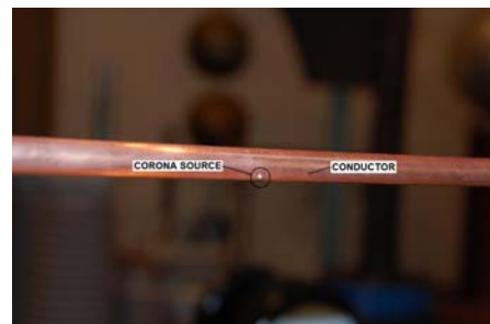
Figure 6: Artificial corona source for space charge measurement experiment
