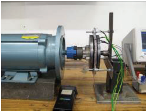
Figure 10: Test configuration with coupled generator and DC motor.
