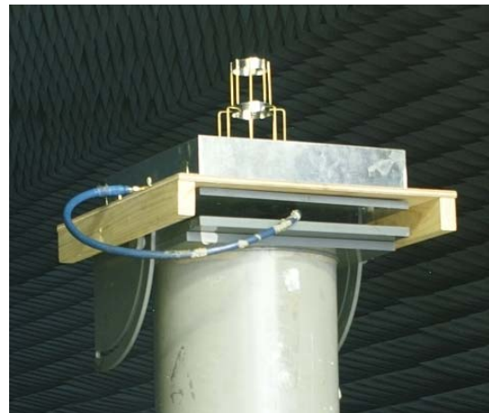
Figure 7: Measurement of second scale model in anechoic chamber
