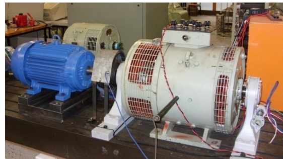
Figure 2: A standard induction motor coupled to a dynamometer in the laboratory
