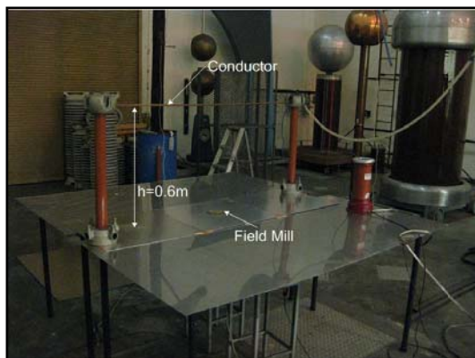
Fig. 13: Experimental setup of wire-plane configuration and sensing electrode flush with ground plane
