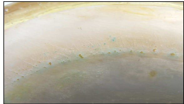
Figure 3: Portion of some of the surface discharge samples showing visible signs of cracks and microvoids after long term (800 hs) ageing under PD activity.
