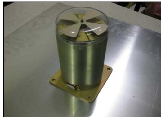
Fig. 5: Developed field mill prototype for E-field measurements
