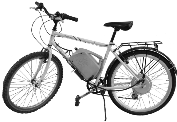
Fig. 10: BLDC controller, battery and BLDC motor fitted to a bicycle.
