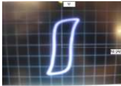
Photo 3.1: Hysteresis loop of a 6 kVA, (230/25) V power transformer operating at nominal voltage
