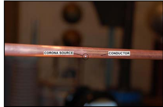
Fig. 14: Smooth copper conductor with artificial corona source
