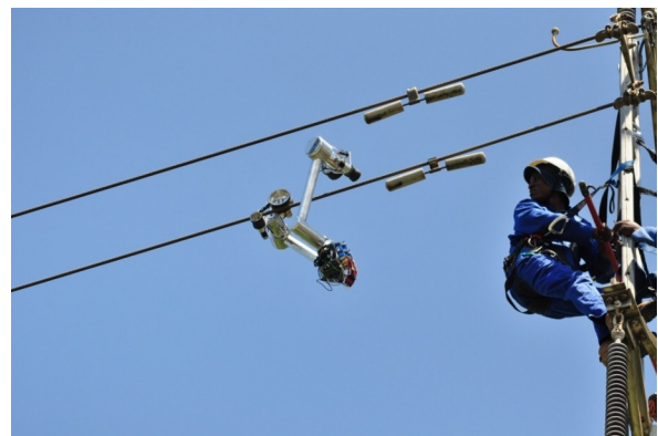
Figure 4: Robot during negotiation of a vibration damper
