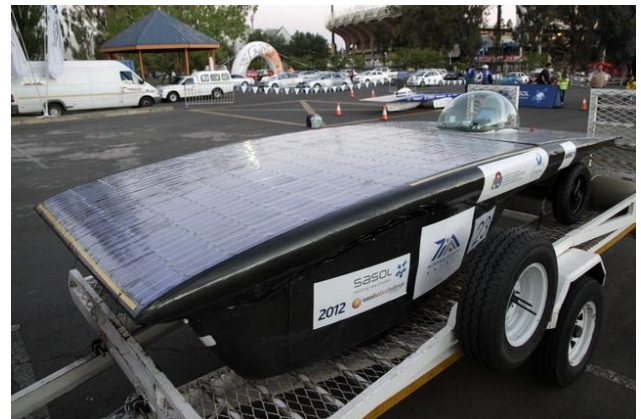
Fig. 1. The NWU solar car containing 252 monocrystalline solar cells.
