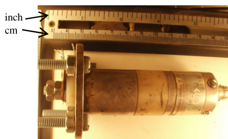
Figure 3: T&M Research Products co-axial current shunt resistor
