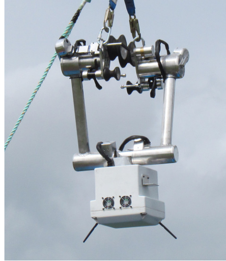
Figure 5: The upgraded robot being winched to the line
