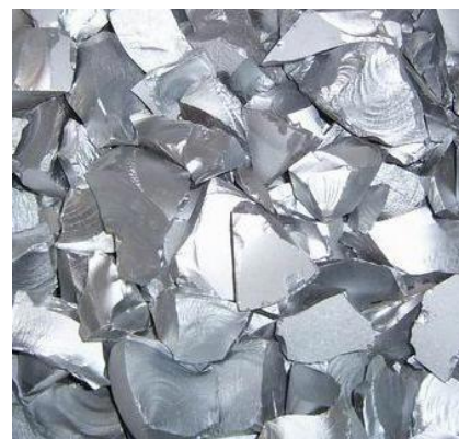
Figure 2: Silicon crystals to be melted [12]
