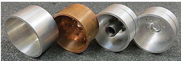
Figure 16: (a) Normal aluminium stator, (b) normal copper stator, (c) equal overhang aluminium stator and (d) zero overhang stator.
