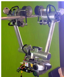
Figure 1: Power Line Inspection Robot developed at UKZN [1].
