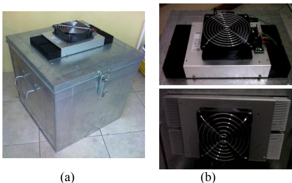
Figure 13: (a) Actual constructed model and (b) AA-100-24-22 thermoelectric heat pumping assembly
