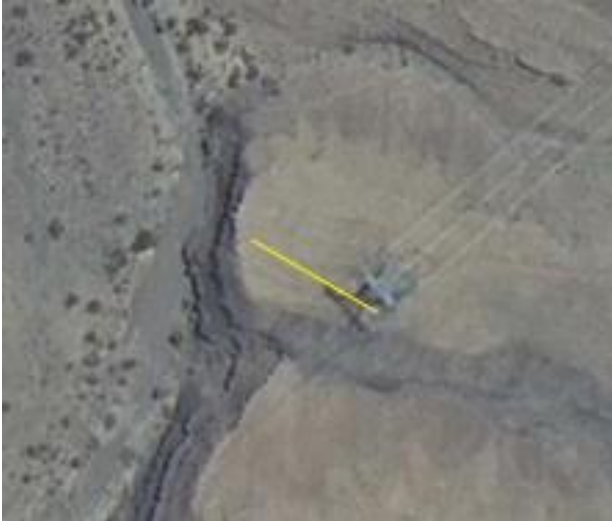
Figure 9: Traverse near the tower of Figure 7 along which soil resistivity measurements were conducted.
