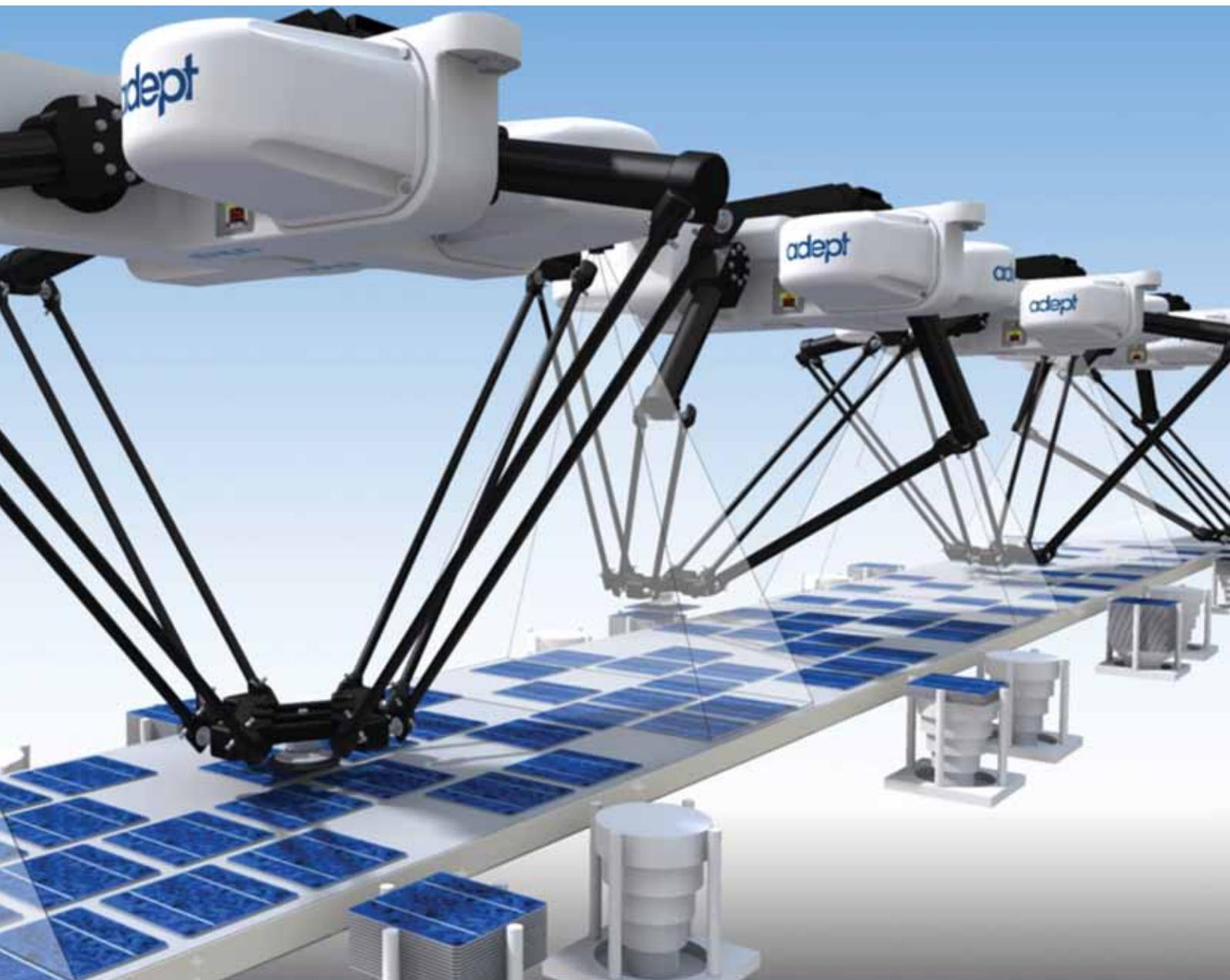
solar cells and even whole modules and then place the gripped objects with great precision and speed.
