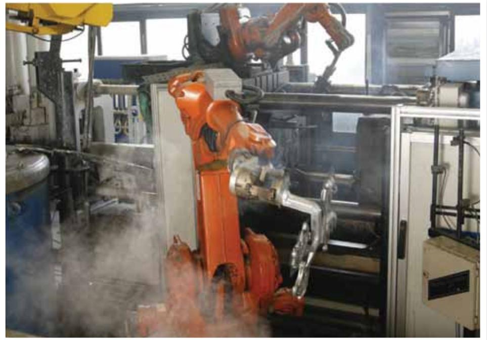
*Two robots work in coordination to remove and deburr the part, then spray the die to prepare for the next drop. This application of robots also removes humans from this high temperature environment*
