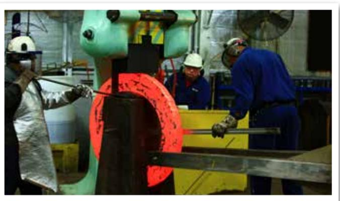
*Open die forging can produce custom prototypes faster than any other forging process.*
