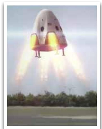
*Simulation of Dragon Landing using its Superdraco rocket engines.*
