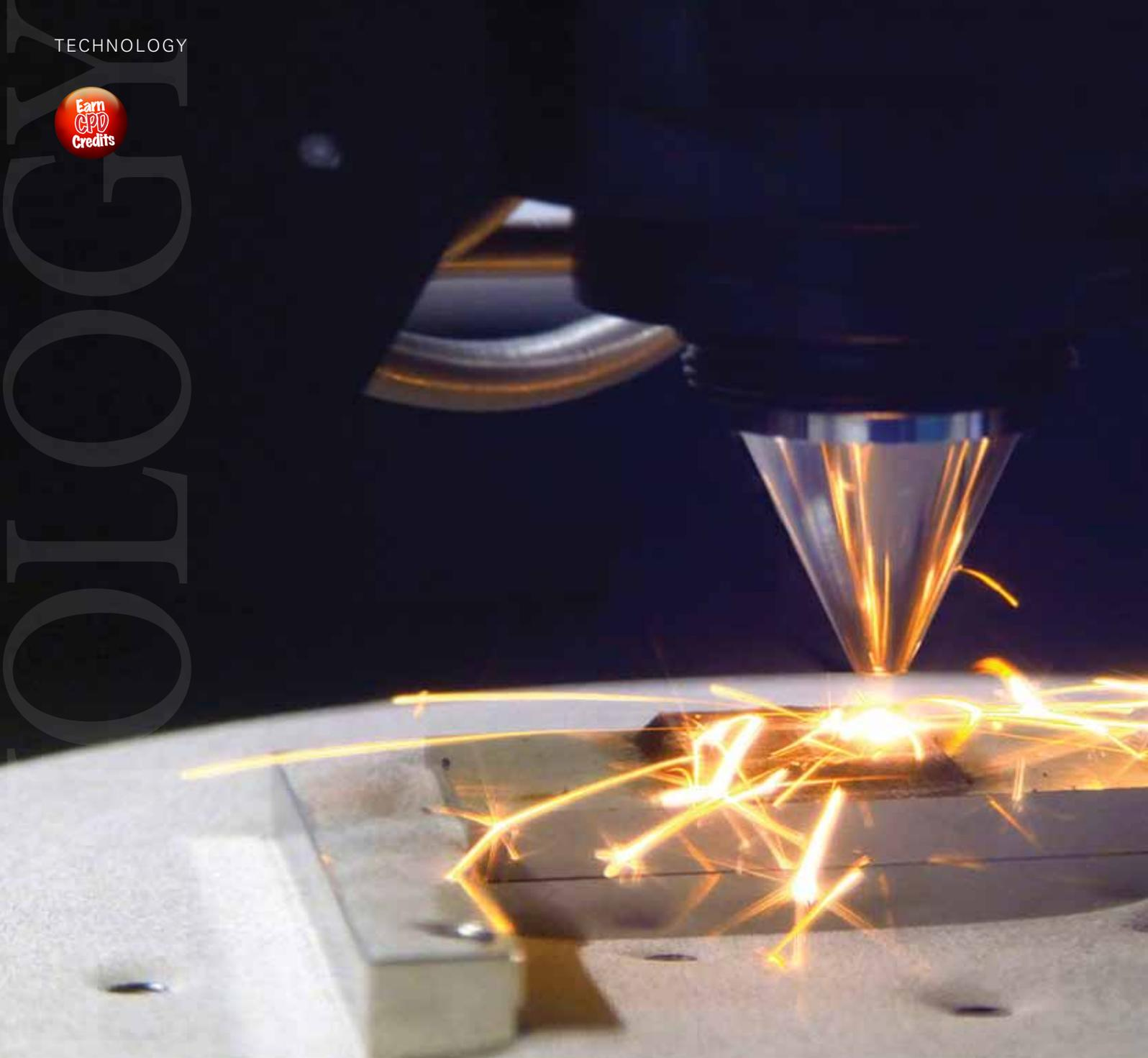
The vast majority of 3D printing technologies focusses on making objects out of plastic, but 3D printing technologies are being developed to build metal objects, generally by laser-sintering powdered metal feedstock. The hope of the universities and corporations pursuing the technique is that the ability to print metal parts will bring about a revolution in industrial production by supplanting traditional metalworking methods like forging.
