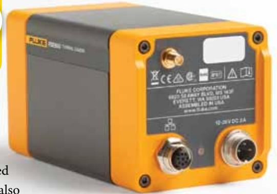
electrical connection, remotely focus the camera, and transmit data and images to PC. Semi-fix the cameras to set up easily repeatable thermal experiments to troubleshoot and improve first pass quality.
