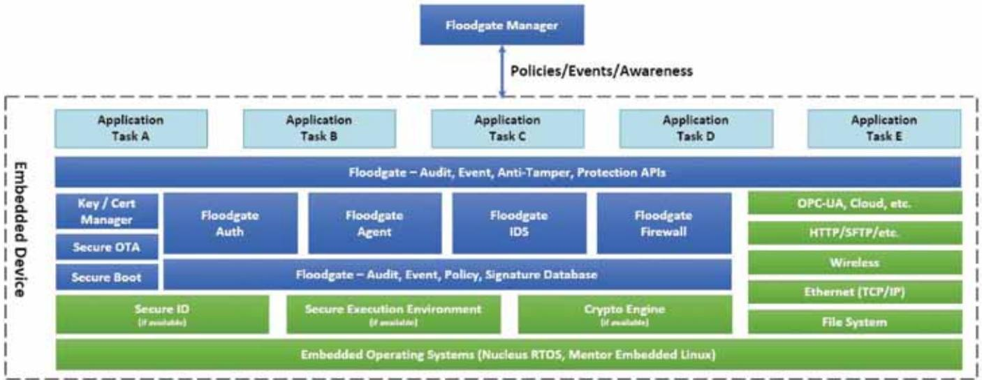
Figure 3: A complete security framework that leverages hardware security features.
