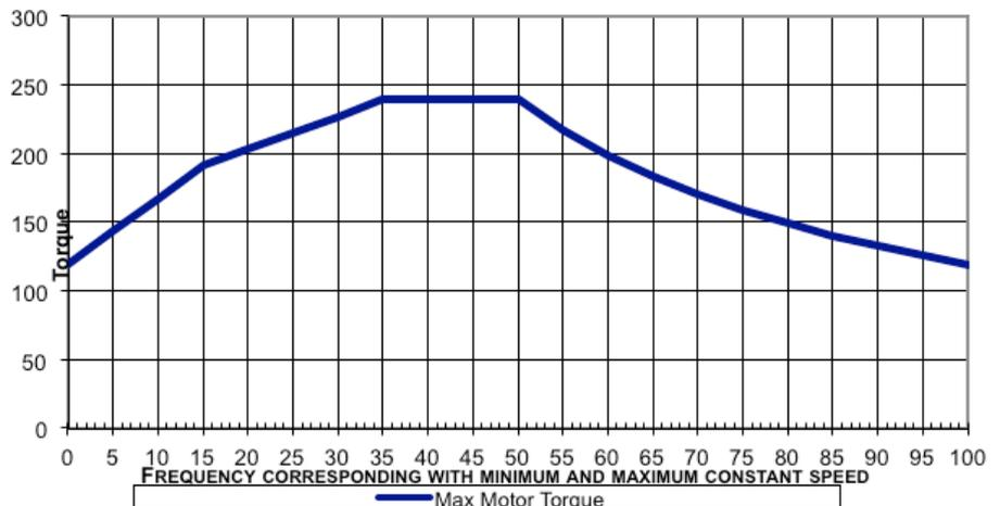
Thermal envelope for VSD driven electric motors
