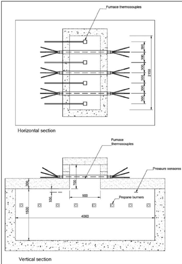
Fig 1 - Furnace setup
