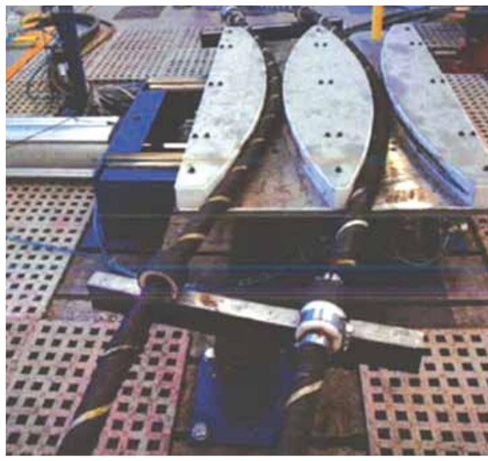
Figure 2: Bending against template test arrangement
