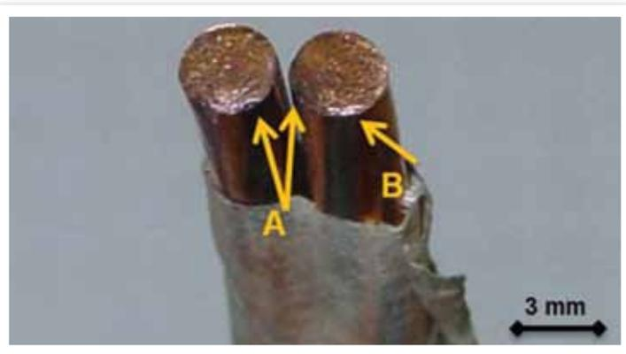
Figure 5: Fatigue failure of a copper conductor wire
