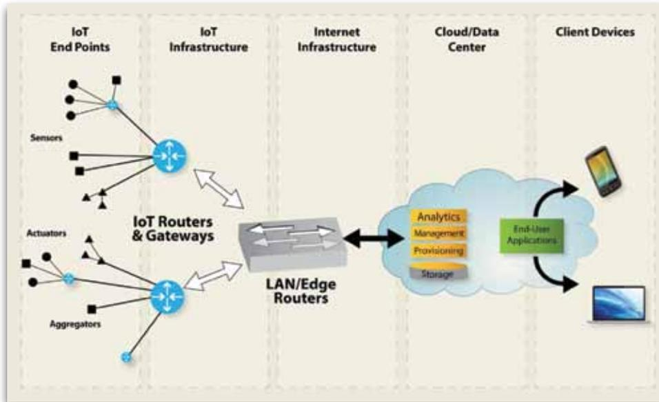
Figure 1: IoT connectivity includes the traditional M2M connected devices, but extends across the network, to the cloud, and beyond.
