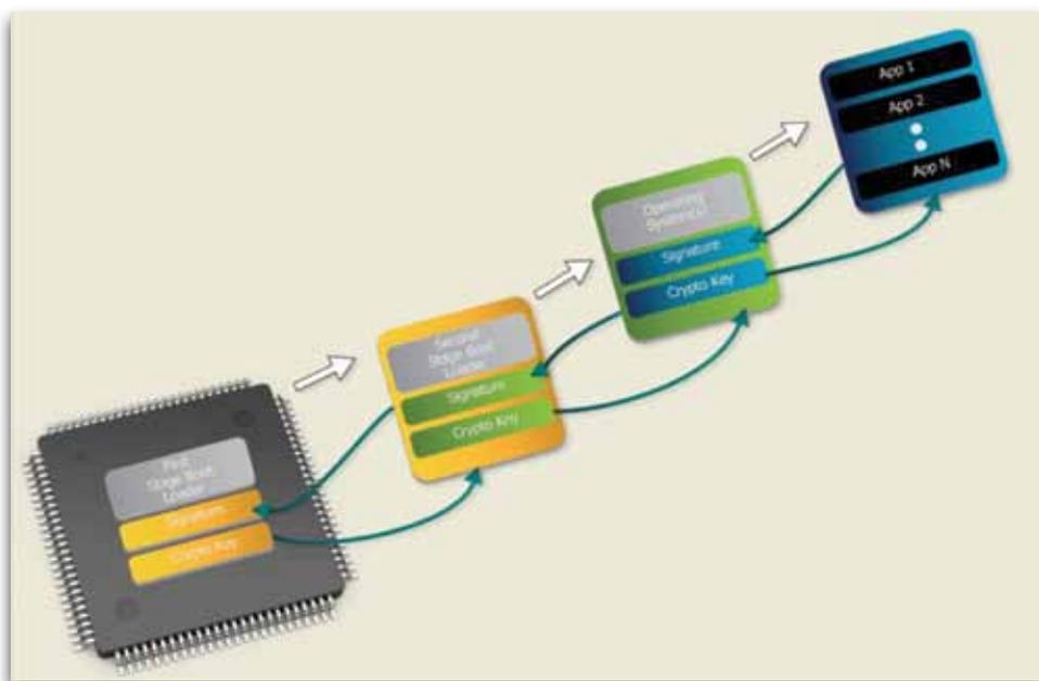
Figure 2: Security requires establishing a chain of trust that begins in the hardware and extends to every bit of software that is loaded on the device.
