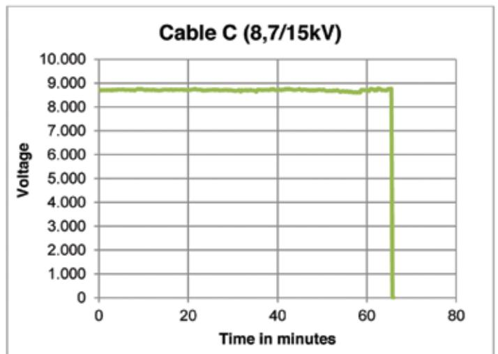
Figure 5: Test result and time breakdown.
