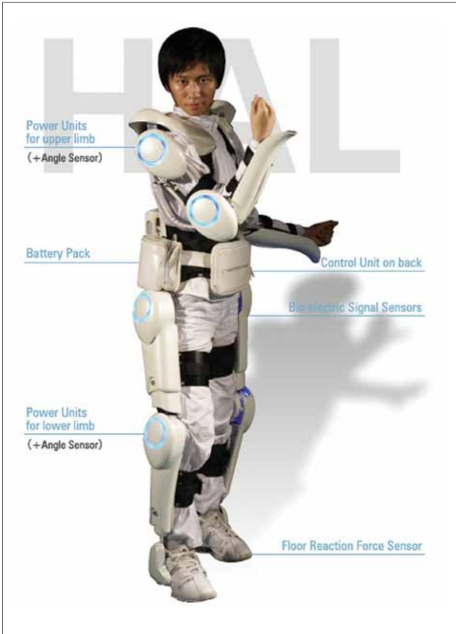
The most exciting is a robotic exoskeleton manufactured by a company called Cyberdyne®. Worse, it's called HAL® (Hybrid Assisted Limb).
