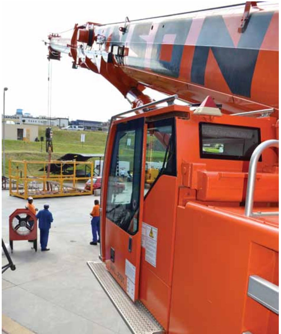
A 275 t Liebherr LTM 1250-6.1 mobile hydraulic crane with a 72m boom was used to hoist the car in its cradle.
