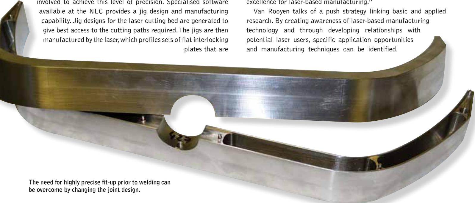
The need for highly precise fit-up prior to welding can be overcome by changing the joint design.
