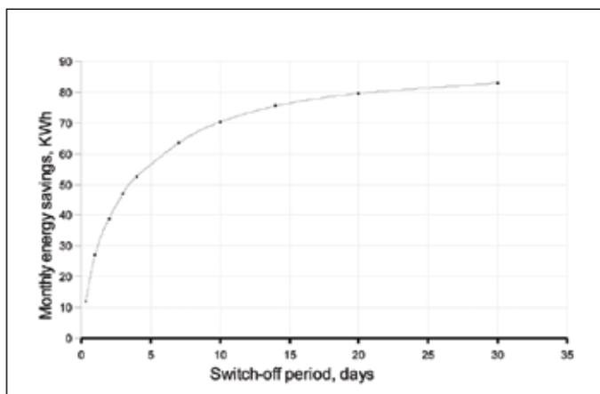
Figure 3: Standby energy saved by switching the geyser off during non-use periods.
