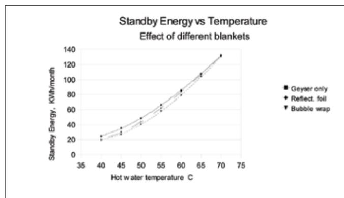
Figure 5: Reduction of standby energy with different geyser blankets.
