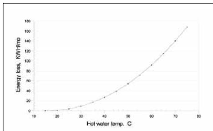
Figure 2: Standby energy of a 150L geyser (derived from cooling curve).
