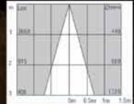
MR16 LED retrofit - source 3 x Cree or Osram LEDs - 350mA driving current
