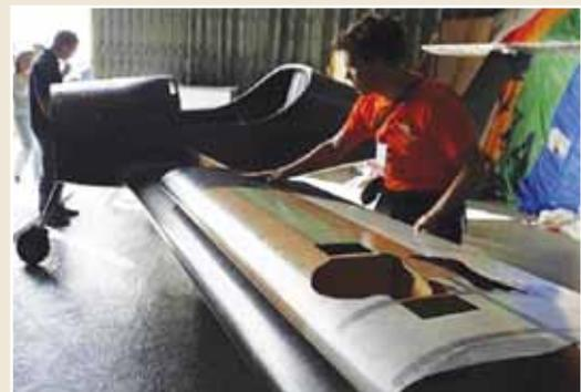
A man places a prototype cork wing on top of the currently-used plastic wing in DynAero's light plane to verify measurements, in a hangar at the Evora airfield September 20, 2009. Image courtesy REUTERS.
