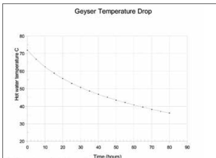
Figure 1: Cooling curve of a 150L geyser (measured).
