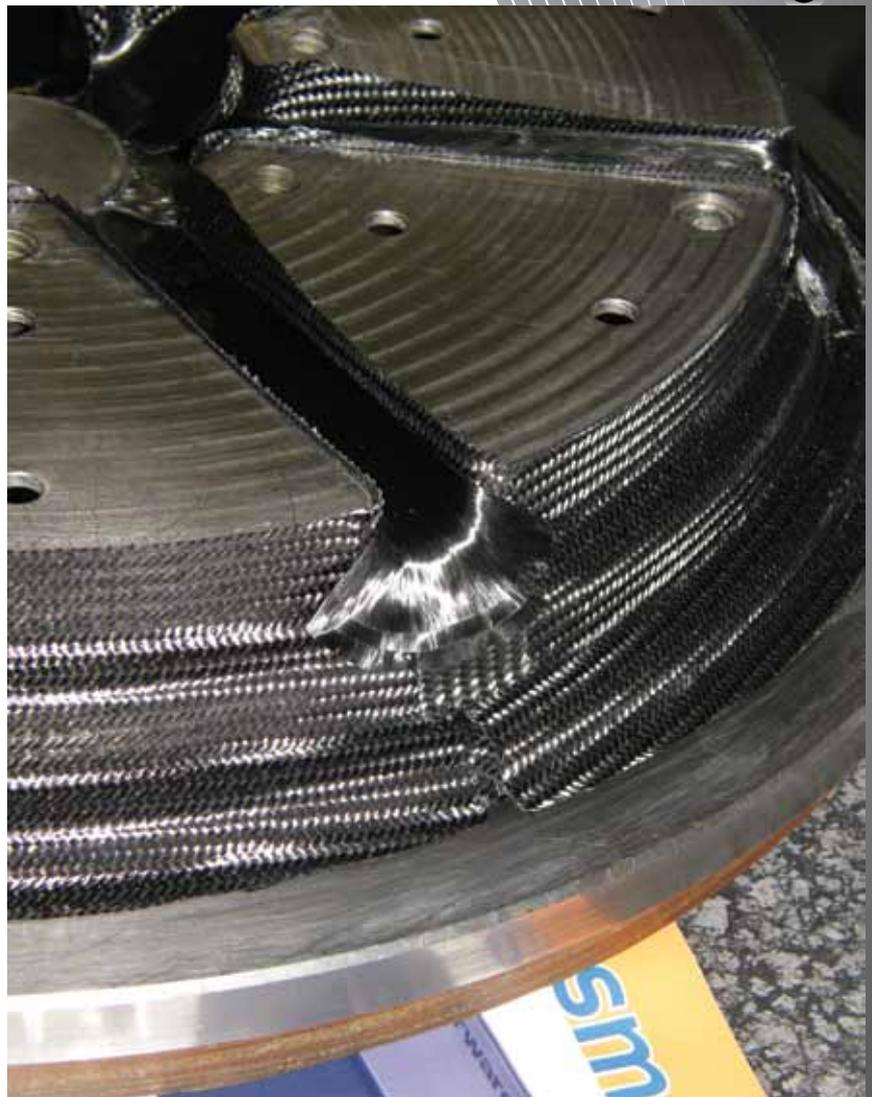
Unidirectional carbon fabric – fanning out from the spokes to join onto the rim – is being laid onto woven fabric layers underneath.
