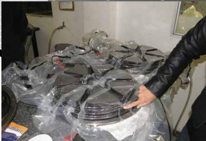
Moulds are placed into vacuum bags for 30 minutes, twice or three times during the layout process to compress/debulk the carbon fibre layers.
