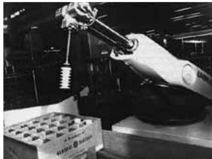
In 1969 Victor Sheinman at Stanford University invented the Stanford arm, an all-electric, six-axis articulated robot designed to permit an arm solution. This allowed the robot to accurately follow arbitrary paths in space and widened the potential use of the robot to more sophisticated applications such as assembly and arc welding.
