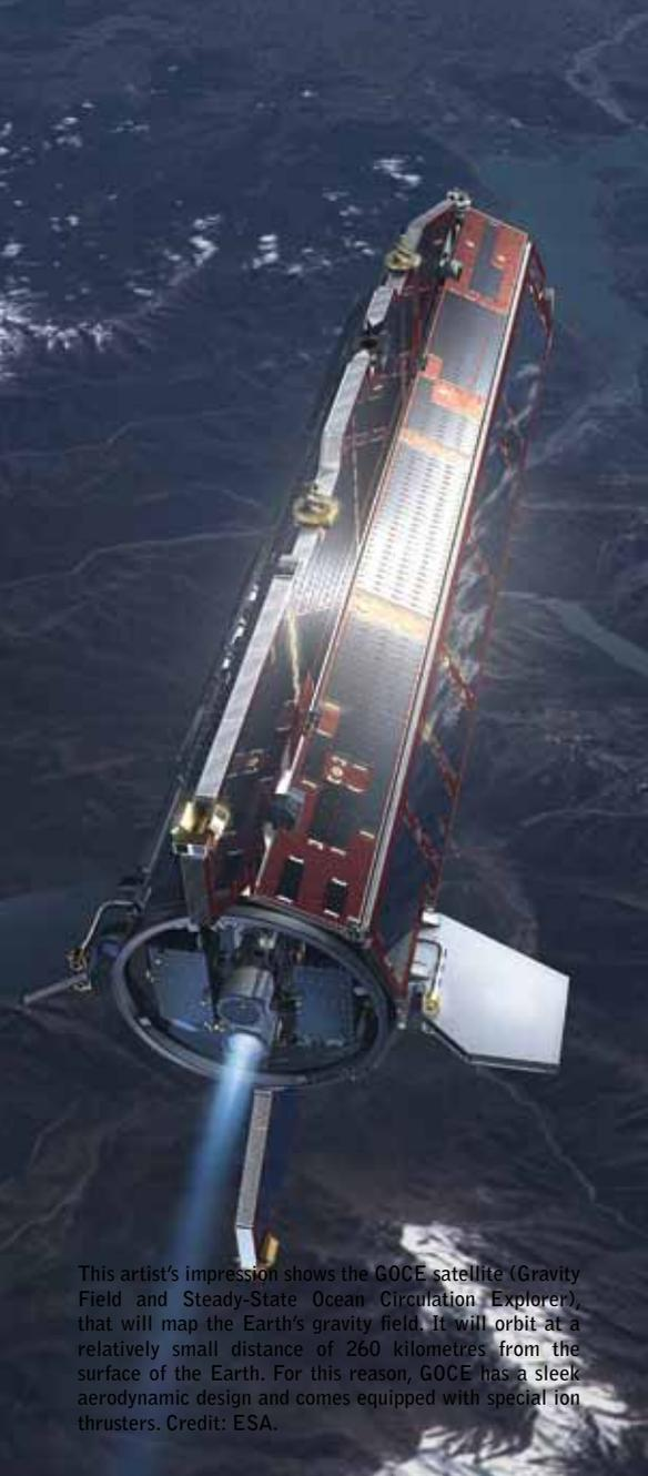
This artist's impression shows the GOCE satellite (Gravity Field and Steady-State Ocean Circulation Explorer), that will map the Earth's gravity field. It will orbit at a relatively small distance of 260 kilometres from the surface of the Earth. For this reason, GOCE has a sleek aerodynamic design and comes equipped with special ion thrusters. Credit: ESA.
