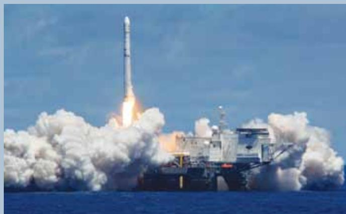
owned by a Russian-led consortium headed by Energia Overseas. Its rig, which operates as the launch pad, and its command ship are located off Long Beach in California but when it is due to launch a payload into space, the rig is towed to the equator at 154 degrees West Longitude.
