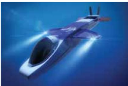
At the moment the craft can carry one crew-member and descend at a rate of 76 metres a minute meaning that a round trip can be done in about five hours. Hawkes and the pilot, Chris Welsh, are currently testing the vessel near Guam.
