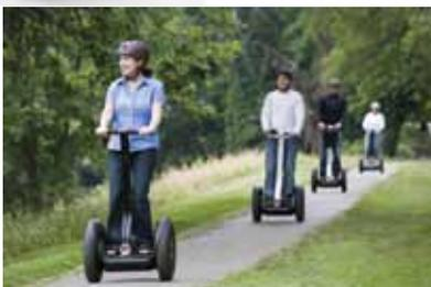
Actuators respond and power the two electric motors responsible for the wheels back and forth to keep a person balanced on top. Lean forward and the device can trot off at about 20 km/h.
