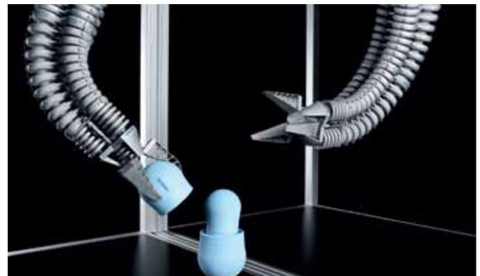
Bionic handling: The Bionic Handling Assistant from Festo offers complete flexibility and the ability to safely move objects from one position to another.
