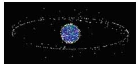
A 'snapshot' of the earth and about 500 of its artificial satellites generated one summer evening in 2002. Nearly all of them are GEOs or LEOs. Satellites on the ring are in geosynchronous earth orbit (GEO). Those clustered near the earth are in low earth orbits (LEO). Scattered in between are satellites in medium earth orbits (MEO). The moon, earth's only natural satellite, is approximately nine times farther from the earth than the ring of geosynchronous satellites. Source: NASA.
