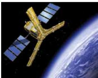
In 2009, the European Space Agency (ESA) launched the Soil Moisture and Ocean Salinity (SMOS) satellite to measure the water content of soil across the planet up to a depth of two metres.
