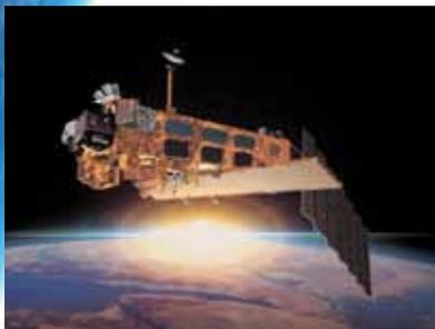
The Earth observation satellite Envisat supplies valuable information about the condition of our planet. The instrument SCIAMACHY (SCanning Imaging Absorption SpectroMeter for Atmospheric CHartographY) onboard Envisat measures the solar radiation scattered back from Earth's surface and atmosphere in the ultraviolet to the near-infrared parts of the spectrum. Credit: ESA.
