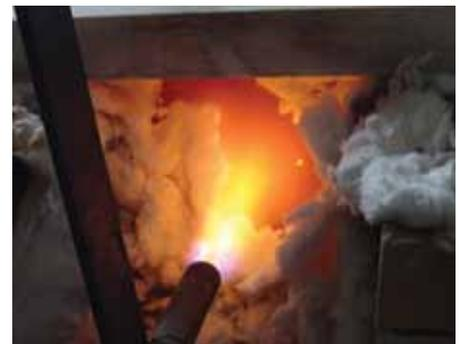
Pyrofoam™ can withstand temperatures up to 1,600°C.
