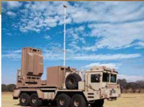
Typical Giraffe surveillance radar (top) suitable for the proposed ground-based air defence launcher system.
