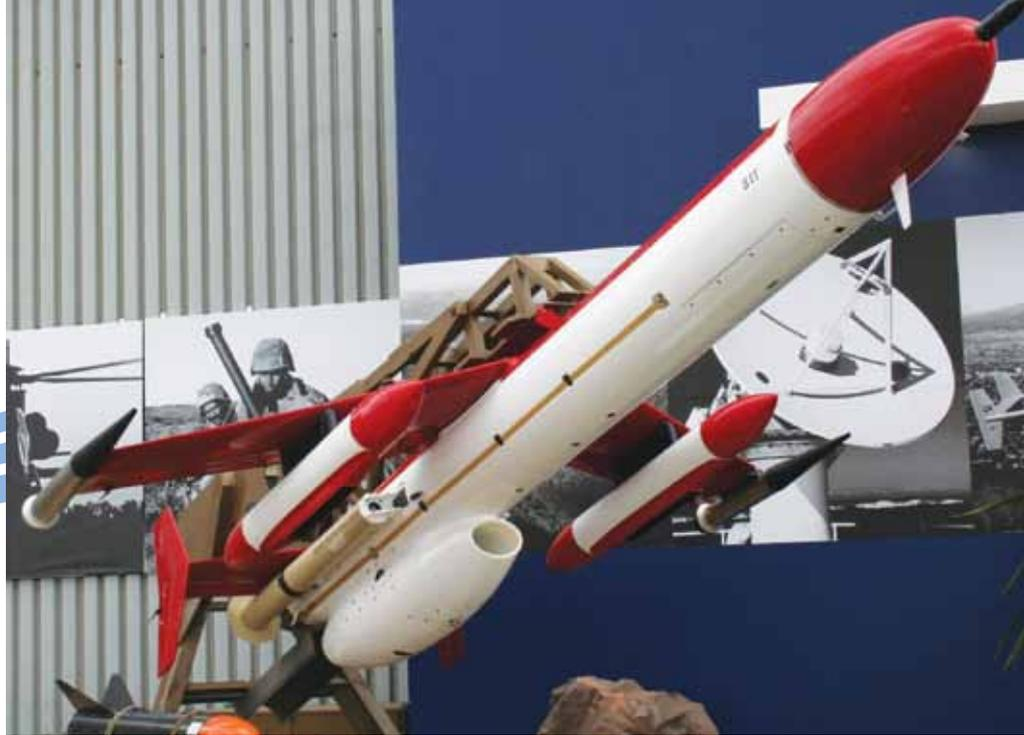
Skua, Denel Dynamic’s high-speed target drone, is designed to simulate high-speed attack aircraft during land, sea and air combat training exercises and weapon development.
