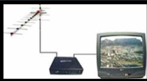
**Figure 3** | DTT reception via an external set-top box receiver interface to an analogue television set
