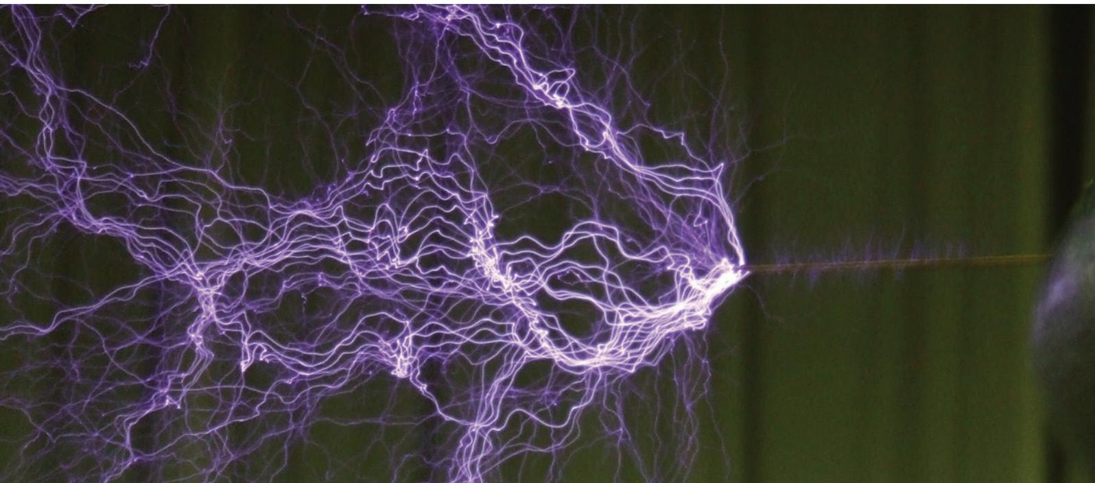
*Plasma discharges from a Tesla coil constricted by Z-pinch*
