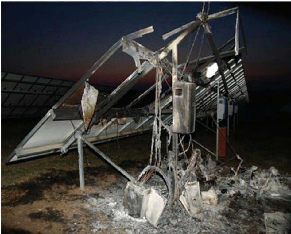
Damaged Solar Plant due to Lightning
